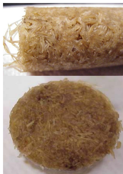
Figure 3. Roots removed from small mist reactor. Final packing density = 0.71; root bed diameter is 2.7 cm. Upper panel is side view; lower panel is cross sectional view of roots half way down the height of the bed.
