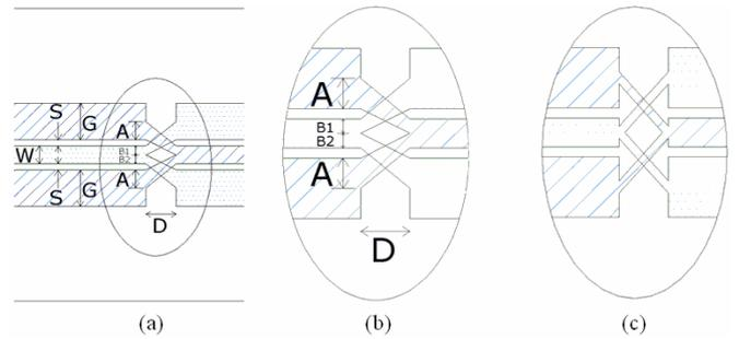
Fig. 4 CPW structure for 180° phase converting (a) Top view (b) Magnified “X”-crossing structure (c) A modified “X”-crossing structure
