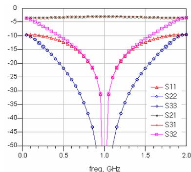
Fig 1. Theoretical characteristics of the basic single stage Wilkinson power divider
