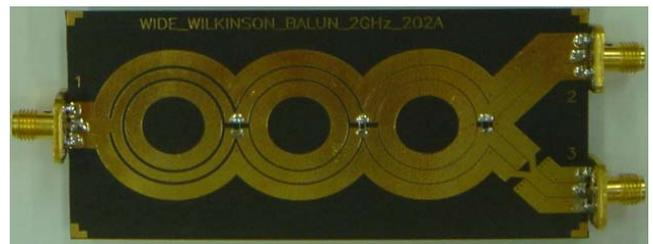
Fig. 7. Fabricated CPW ultra-wide band balun.
