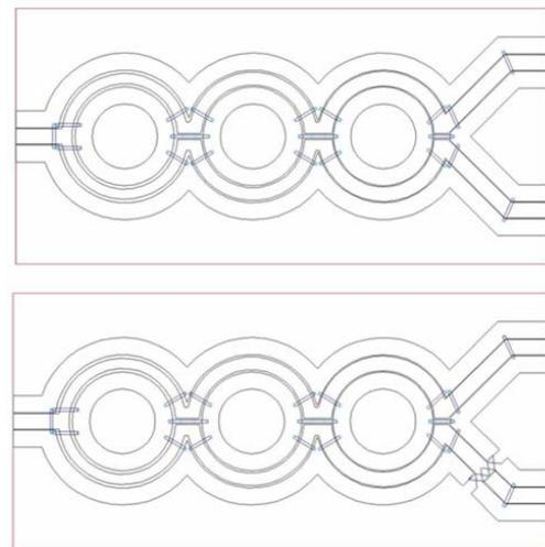
Fig. 6. Layouts of the CPW 3-stage ultra-wide band Wilkinson divider and balun (substrate thickness = 31mils, dielectric constant=2.2)
