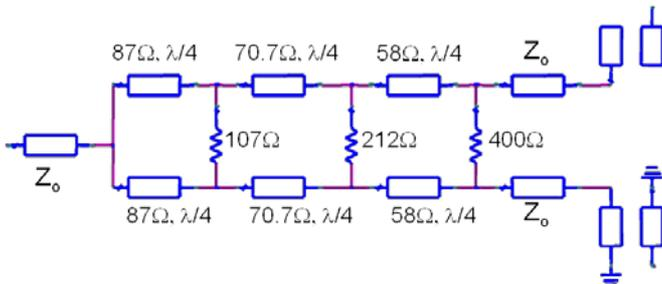
Fig. 3. Balun with the wide band Wilkinson divider and couplers
