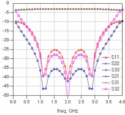
Fig. 2. Theoretical characteristics of a 3-stage Wilkinson divider
