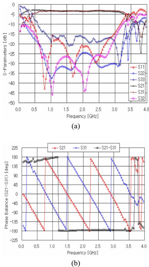
Fig. 8. Measured data of the 3-stage ultra-wide band CPW balun (a) S-parameters (b) phase
