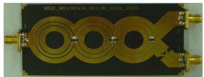
Fig. 7. Fabricated CPW ultra-wide band balun.
