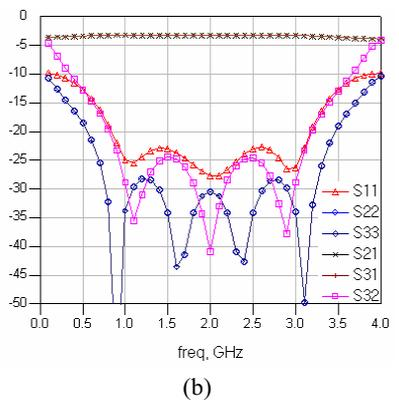
Fig. 5. (a) 3-stage ultra-wide band CPW balun (b) Ideal S-parameters (c) Ideal phase characteristics
