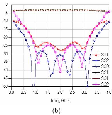
Fig. 5. (a) 3-stage ultra-wide band CPW balun (b) Ideal S-parameters (c) Ideal phase characteristics
