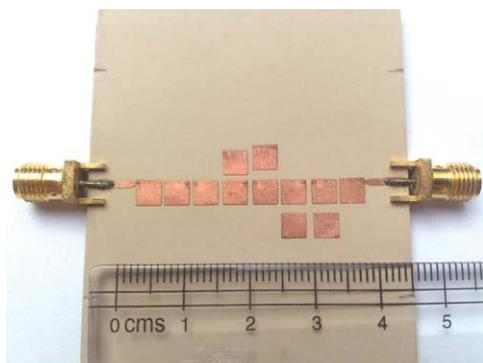
Figure 9 Fabricated picture of triple-bandpass filter using metamaterial mushroom resonators.
