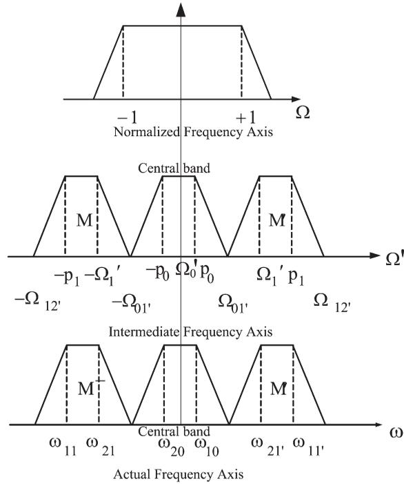
**Figure 1** Frequency response of the filter in three different frequency domains,  $\Omega$  is the normalized frequency for a single-passband low-pass prototype and  $\Omega'$  is the normalized frequency for a triple-passband filter. The  $\omega$  domain is the actual frequency domain where the filter operates [9, 12].
