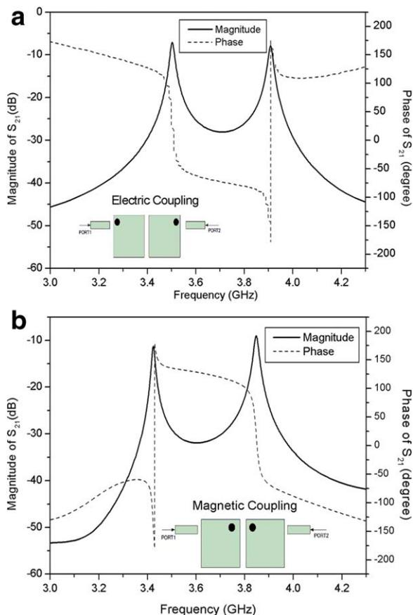
**Figure 5**  $S_{21}$  response of weakly coupled mushroom structure. (a) Electric coupling. (b) Magnetic Coupling.
