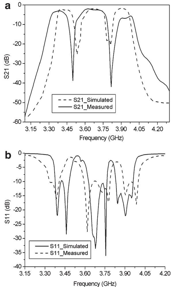
**Figure 8** EM simulated/measured results of triple bandpass filter. (a)  $S_{21}$ , (b)  $S_{11}$ .
