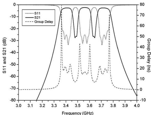
**Figure 4** Frequency response of S11/S21 and group delay in circuit simulation.
