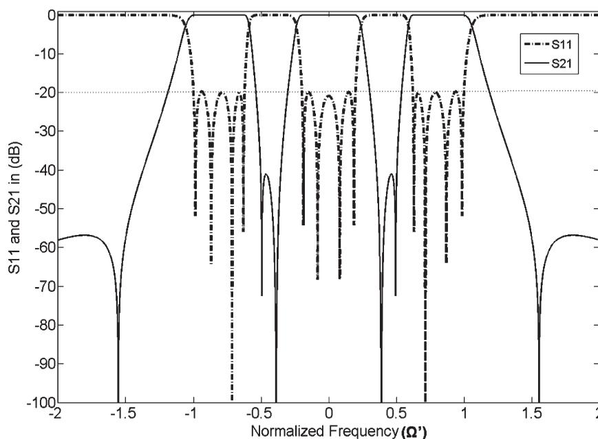
**Figure 2** Theoretical response of 12-pole triple bandpass filters from the coupling matrix [transmission zero at  $s = \pm j2.0, c_1 = 0.40, c_1' = 1.5$  and  $c_0 = 0.2, RL 20 \text{ dB}$ ].
