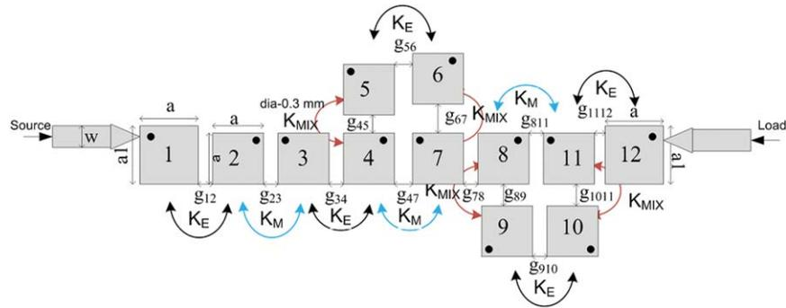
**Figure 7** Triple-band filter layout [ $a = 4$ ,  $a1 = 4.1$ ,  $W = 1.13$ ,  $g_{12} = g_{1112} = 0.36$ ,  $g_{23} = 0.58$ ,  $g_{34} = 0.66$ ,  $g_{45} = 0.83$ ,  $g_{56} = 0.73$ ,  $g_{67} = 1.62$ ,  $g_{47} = 0.86$ ,  $g_{78} = 0.5$ ,  $g_{89} = g_{1011} = 1.43$ ,  $g_{910} = 0.95$ ,  $g_{811} = 0.89$ ,  $g_{1112} = 1.58$ , via diameter = 0.3, all dimensions are in mm].
