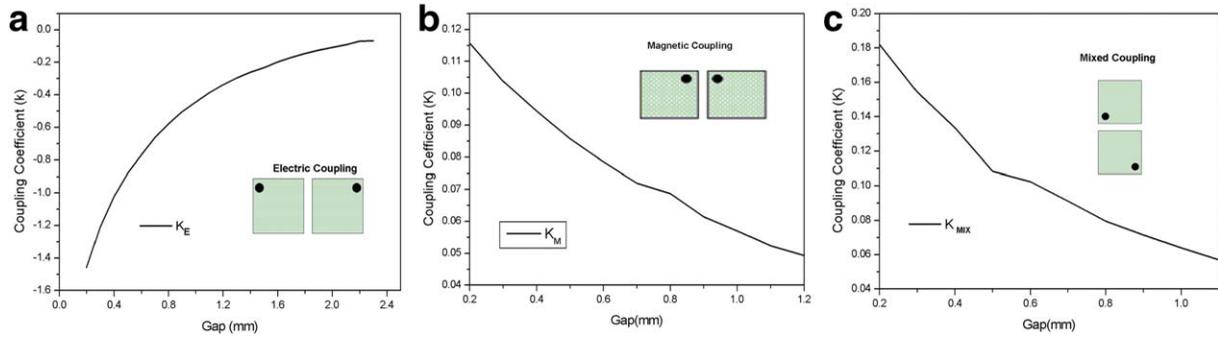
**Figure 6** Mapping of the different coupling coefficients as a function of the distance (gap) between coupled mushroom resonators. (a) Electric coupling  $K_E$ . (b) Magnetic coupling  $K_M$ . (c) Mixed coupling  $K_{MIX}$ .
