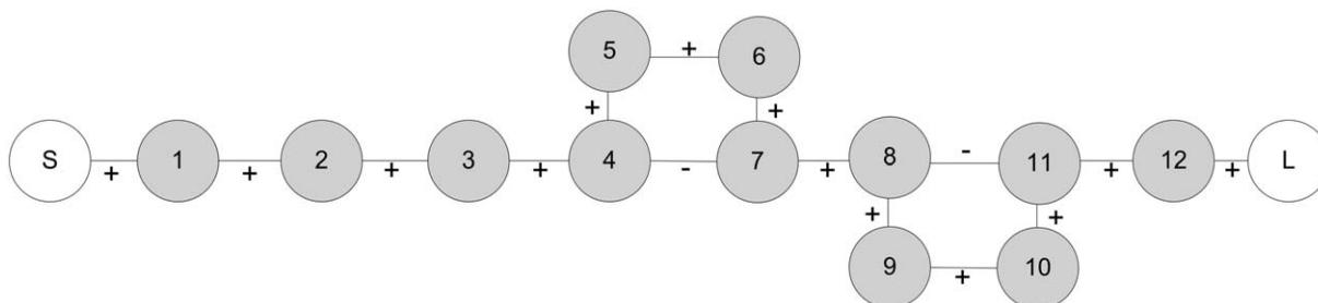
Figure 3 Coupling and routing diagram of 12-pole triple bandpass filter.
