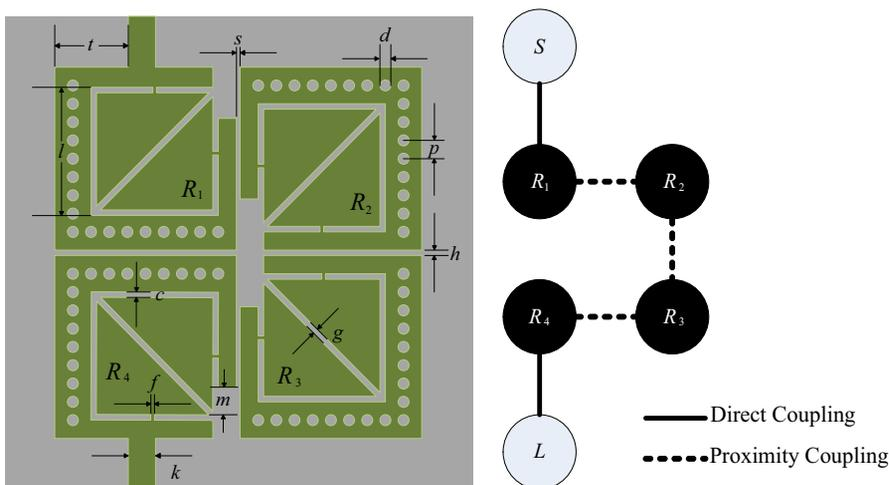
Figure 10. The proposed CQ filter and its general coupling structure.
