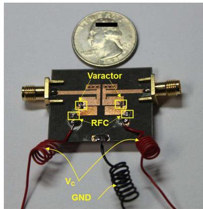
**Figure 5.** Fabricated reconfigurable microstrip LC bandpass filter based on semiconductor varactor diode.
