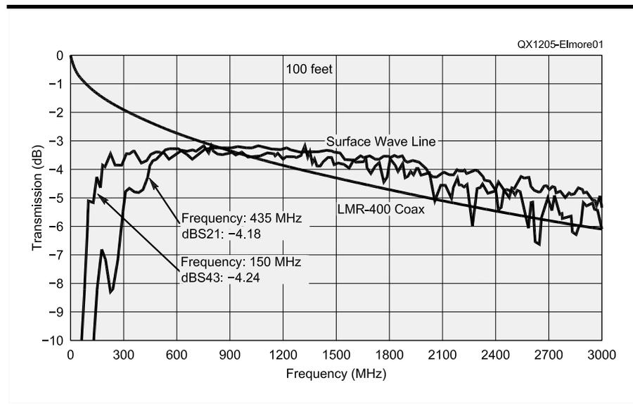
**Figure 1 — Measured performance of SWTL compared with measurement of Times Microwave LMR-400 coaxial cable. Plots of 100 feet of no. 24 AWG conductor with a pair of 400 MHz launchers and a pair of 144 MHz launchers are shown. The main difference between these is the cut-off frequency.**
