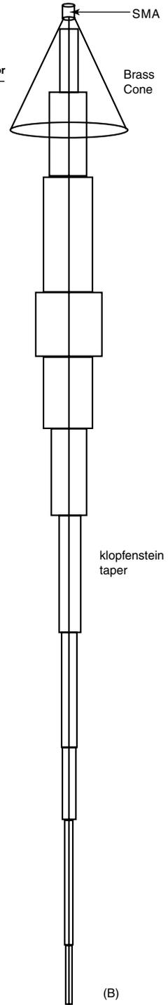
Figure 2 — Part A shows the metalized paper and brass shim stock cone patterns before folding. Part B gives the dimensions of the inner launcher tapered conductor sections made from K&S Metals brass tubing (in 32nds of an inch) versus position from the SMA connector for the 400 MHz launcher.
