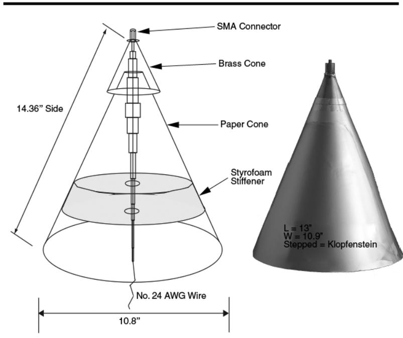
Figure 3 — Assembly of the 400 MHz Launcher.
