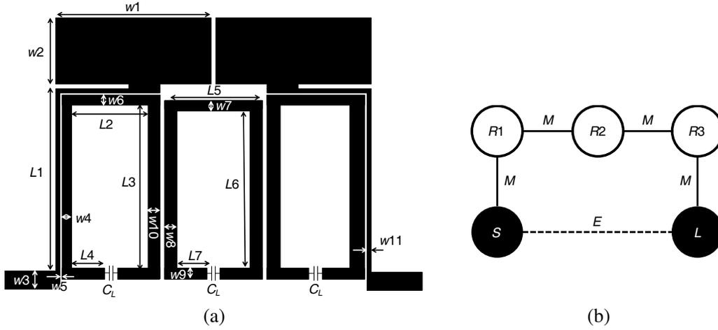
**Figure 1.** The proposed third order tunable filter: (a) the configuration, (b) the coupling topology.
