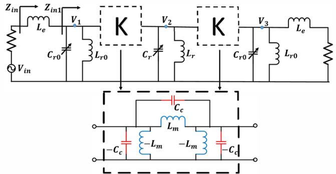
Figure 1. Circuit schematic of a third-order bandpass filter. The inter-resonator couplings K are realized with a mixed electric/ magnetic scheme that is actualized with a parallel LC (represented by  $C_c$  and  $L_m$ ) resonator. The external coupling is realized by means of inductive elements (represented by  $L_e$ ).
