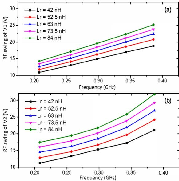
Figure 4. RF swing on different resonator nodes of the filter architecture in Figure 1 for a 10 V AC input voltage. Note that the voltage at node V3 is the same as the voltage at node V1 for various levels of  $L_r$ . Furthermore, the indicated RF swing corresponds to tunable BPF responses that cover the same tuning range and feature constant BW of 55 MHz.
