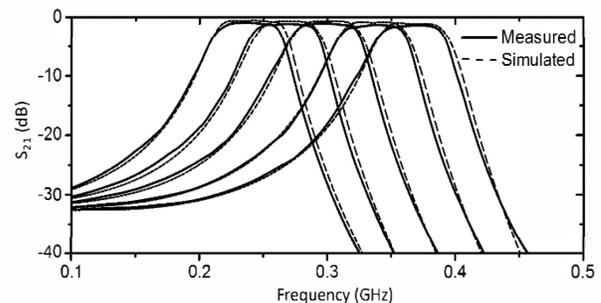
Figure 7. Transmission response of the tunable third-order bandpass filter: RF-measured and ADS simulated.
