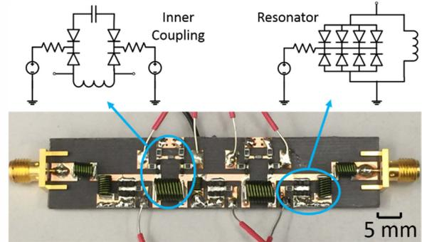
Figure 6. Manufactured prototype of the third-order lumped-element filter with variable center frequency and constant absolute bandwidth.
