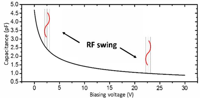
Figure 3. C-V curve of a PIN-varactor with  $n=0.5$
