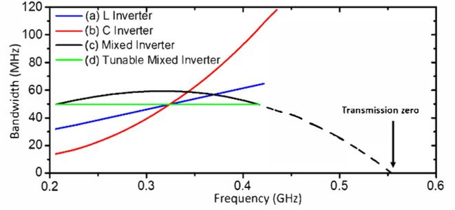
Figure 2. Filter bandwidth as a function of frequency for alternative inter-resonator coupling schemes.
