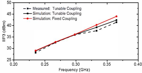
Figure 8. Measured and simulated IIP3 versus filter center frequency.
