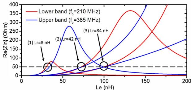
Figure 5. Input impedance of the filter architecture in Figure 1 for various levels of  $L_r$ ,  $L_e$  for the two extreme tuning state in which the BPF is located at 210 MHz and at 385 MHz.
