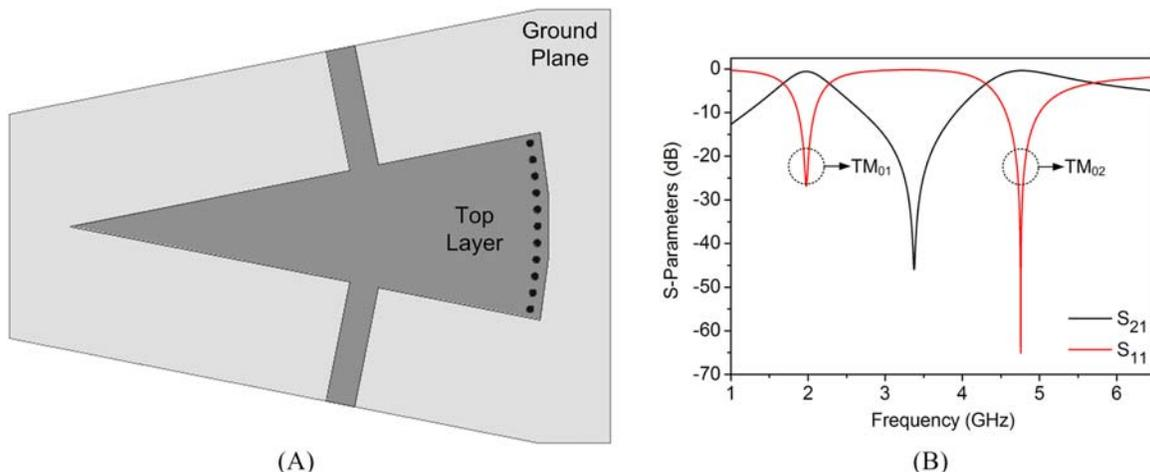
**FIGURE 3** (A) Single cavity structure; (B) Simulated frequency response. [Color figure can be viewed at wileyonlinelibrary.com]
