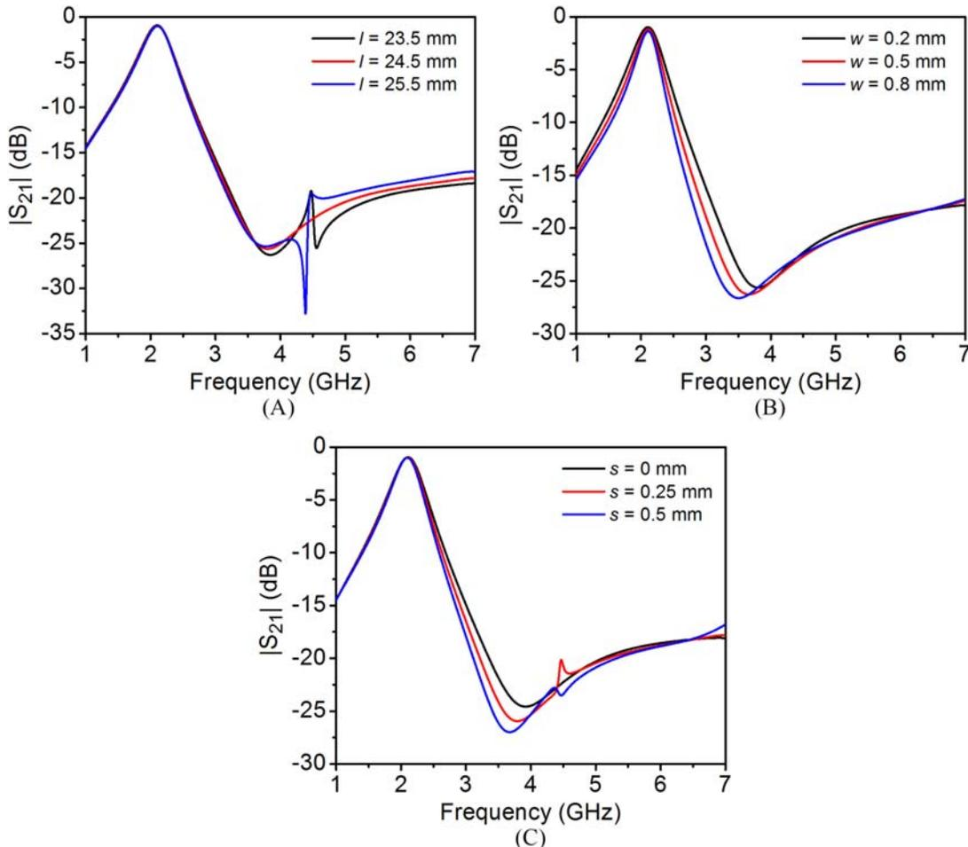
FIGURE 5 Simulated frequency response against (A)  $l$ ; (B)  $w$ ; (C)  $s$ . [Color figure can be viewed at wileyonlinelibrary.com]
