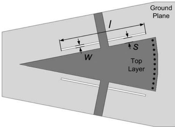
FIGURE 4 Single cavity with ground slots
