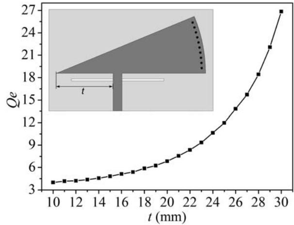
FIGURE 6 External quality factor  $Q_e$  against position of the feedline  $t$
