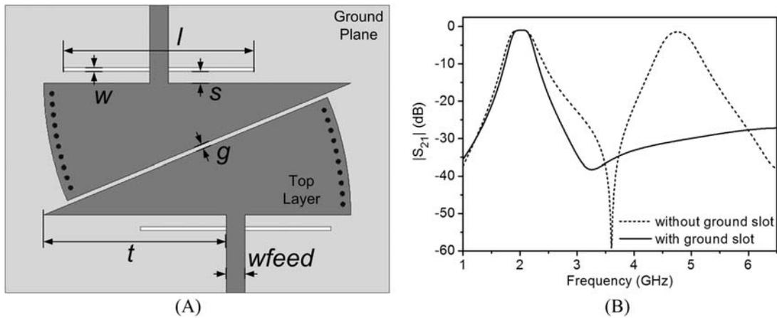
FIGURE 8 (A) Two-pole bandpass filter with slots on ground plane; (B) Comparison of  $|S_{21}|$  (dB) of bandpass filters with and without slots on ground plane
