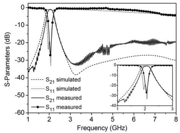
FIGURE 10 Simulated and measured filter response
