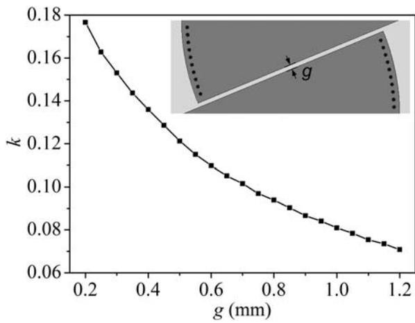
FIGURE 7 Coupling coefficient against  $g$
