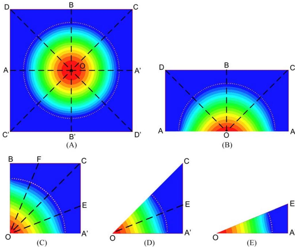
**FIGURE 1** Simulated electric field distributions: (A) Full-mode SIW; (B) Half-mode SIW (HMSIW); (C) Quarter-mode SIW (QMSIW); (D) Eighth-mode SIW (EMSIW); (E) Sixteenth-mode SIW (SMSIW). [Color figure can be viewed at [wileyonlinelibrary.com](http://wileyonlinelibrary.com)]
