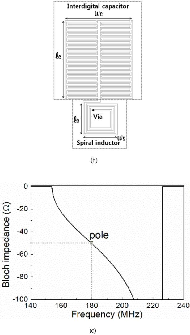
Figure.1. Equivalent circuit, geometry of the CRLH-TL unit-cell, and representative characteristic ( $l_s = 4.7$ ,  $l_c = 10.36$ ,  $w_s = 4.7$ ,  $w_c = 9.16$ , unit: mm) (a) Equivalent circuit (b) Physical shape of the CRLH-TL unit cell (c) Bloch impedance.
