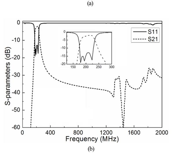
Figure. 2. Geometry of the proposed VHF bandpass filter and its frequency response (a) Physical shape (b)  $S_{11}$  and  $S_{21}$ .
