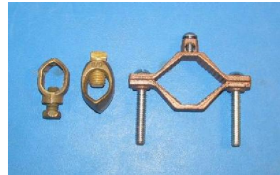
Fig. 16 – Ground rod clamps. The two clamps on the left are for copper-clad steel ground rods and can accommodate a single grounding electrode conductor. The clamp on the right is used for connection to galvanized pipe or conduit such as a mast or water pipe
