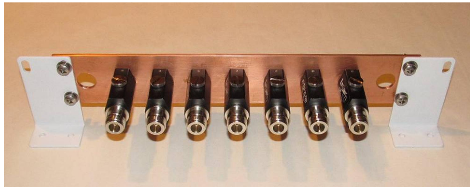
lightning arrestors shown use type N connectors and provide the means to bond the cable shields to ground
