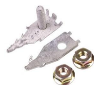
Fig. 9 – Shield bond connector (also called “bullet-bond”). Variations of these are available for use with different cable diameters. The two pieces are slipped between the cable jacket and shield and between the shield and cable core and then are clamped with one nut. The other nut holds the ring lug on the bonding conductor
