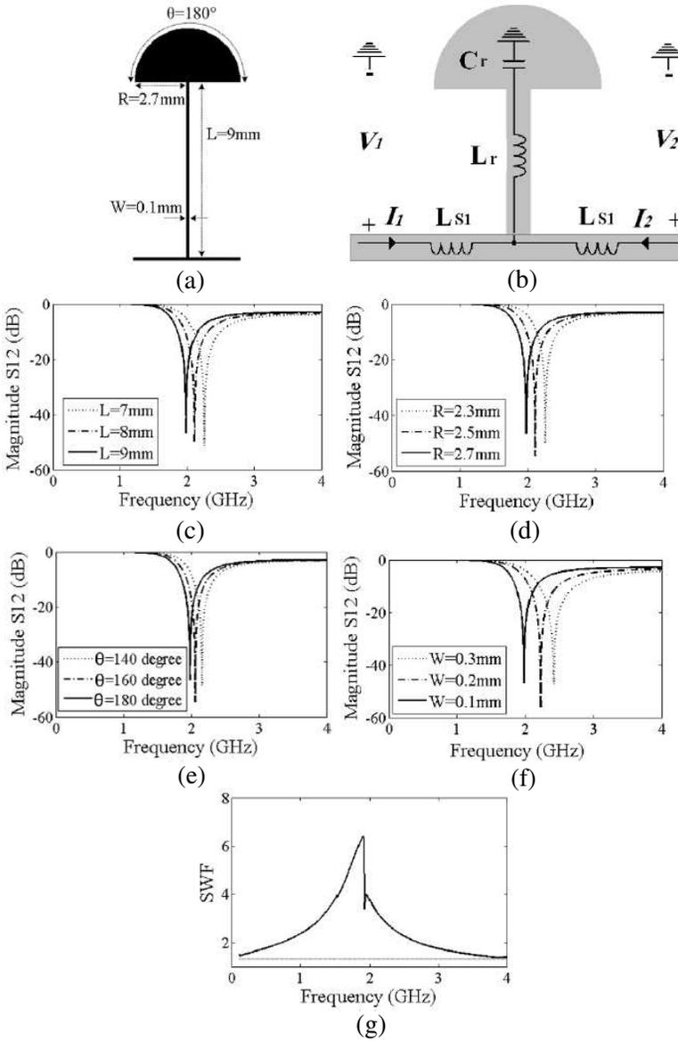
**Figure 1.** (a) Typical topology of proposed resonator. (b) LC equivalent circuit of the proposed resonator. (c) Simulated  $S_{21}$  parameter as function of  $L$ . (d) Simulated  $S_{21}$  parameter as function of  $R$ . (e) Simulated  $S_{21}$  parameter as function of  $\theta$ . (f) Simulated  $S_{21}$  parameter as function of  $W$ . (g) The slow wave factor of the proposed resonator.
