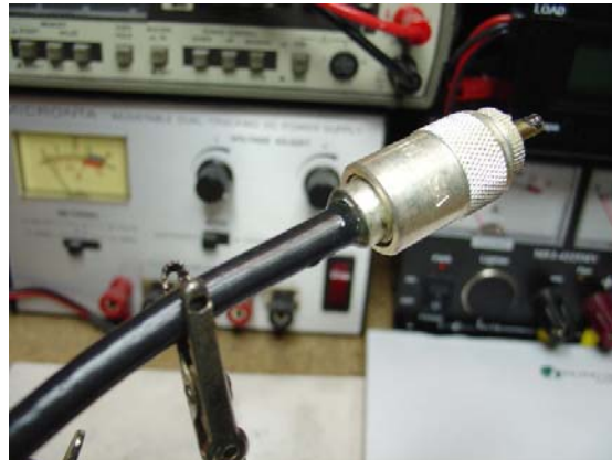
Completed connector with epoxy
