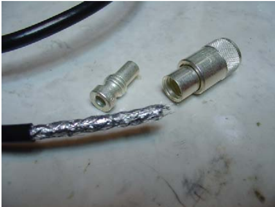
Ready to pull through the reducer
