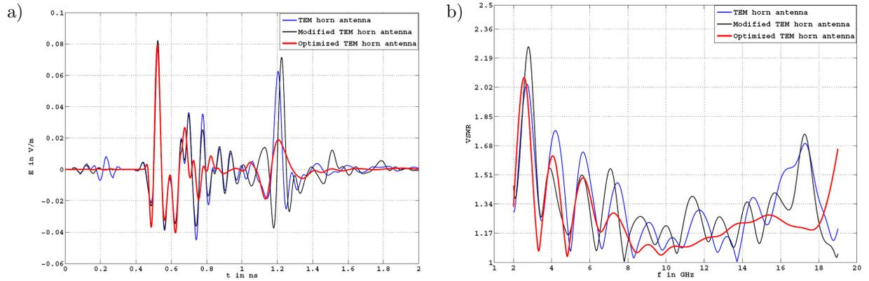
Figure 2: Comparison of different TEM horn antennas: (a) time domain characteristics; (b) VSWRs
