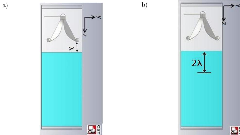
Figure 3: GPR scenarios: (a) empty earth half-space; (b) a scatterer embedded in the earth half-space
