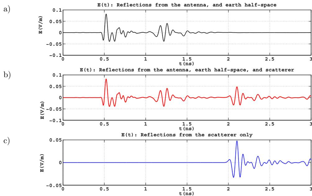
Figure 4: Computed reflections: (a) empty earth half-space; (b) earth half-space with scatterer; (c) scattered field
