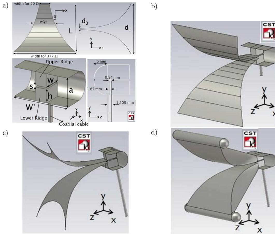
Figure 1: TEM horn antenna: (a) design paramters; (b) original, (c) modified, and (d) optimized geomerty
