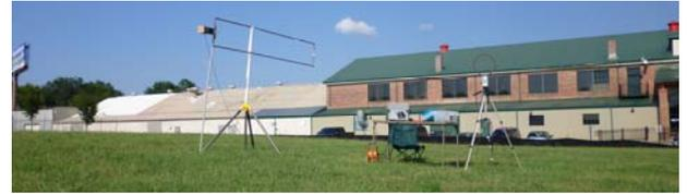
Fig. 11. Testing a 3m 450ohm quadrupole antenna (Trials #1 and #2).
