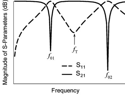
Fig. 2. Typical frequency response of the DGS that exhibit multi stop bands.
