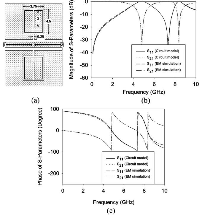
Fig. 4. (a) Layout of the CPW DGS modeled. (b) Magnitude and (c) phase responses of theoretical (circuit model) and full-wave EM (Sonnet *em*) results.
