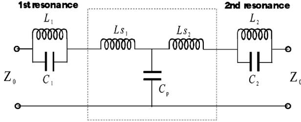
Fig. 3. General circuit model for the DGS.
