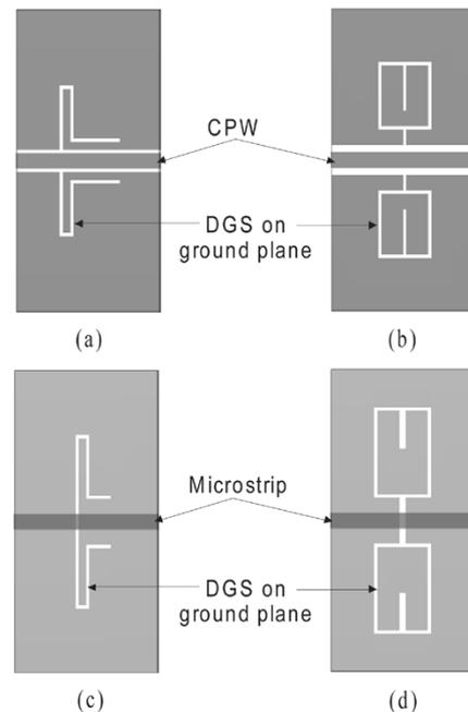
Fig. 1. Various defected ground structures: (a) CPW L-shaped DGS, (b) CPW metal-loaded dumbbell-shaped DGS, (c) microstrip L-shaped DGS, and (d) microstrip metal-loaded dumbbell-shaped DGS.
