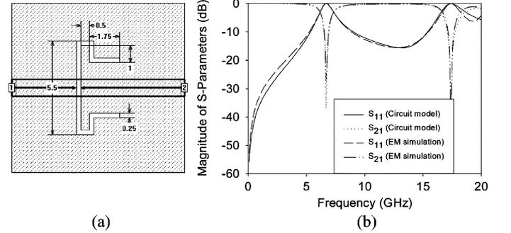
Fig. 5. (a) Layout of the microstrip DGS modeled. (b) Magnitude responses of theory (circuit model) and full-wave EM simulation.
