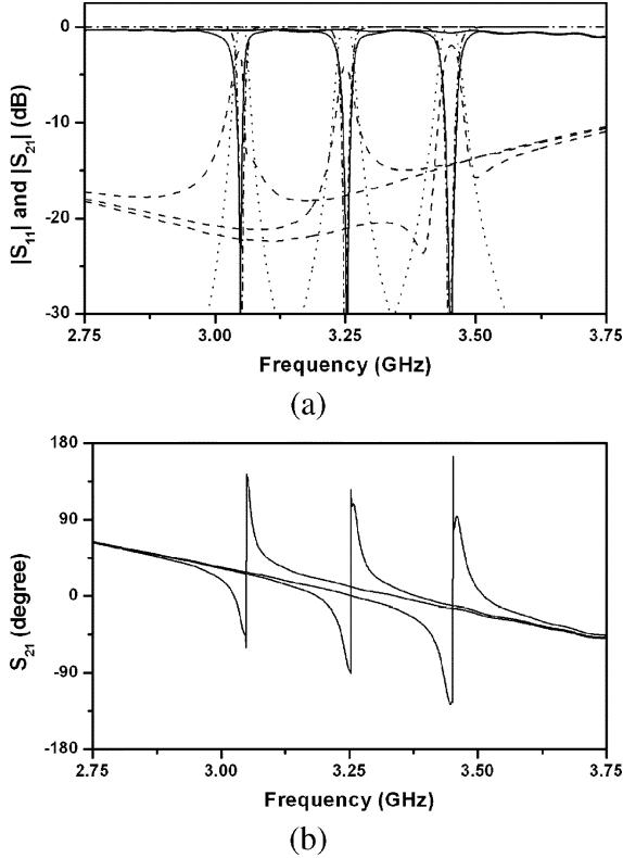
Fig. 3. Measured frequency response of the fabricated bandstop filter. The filter is tuned to exhibit Butterworth bandstop responses at three different center frequencies: (a)  $|S_{11}|$  measurement (— —),  $|S_{21}|$  measurement (— —),  $|S_{11}|$  synthesis (· · ·),  $|S_{21}|$  synthesis (— — —), (b)  $S_{21}$  (degree) measurement.
