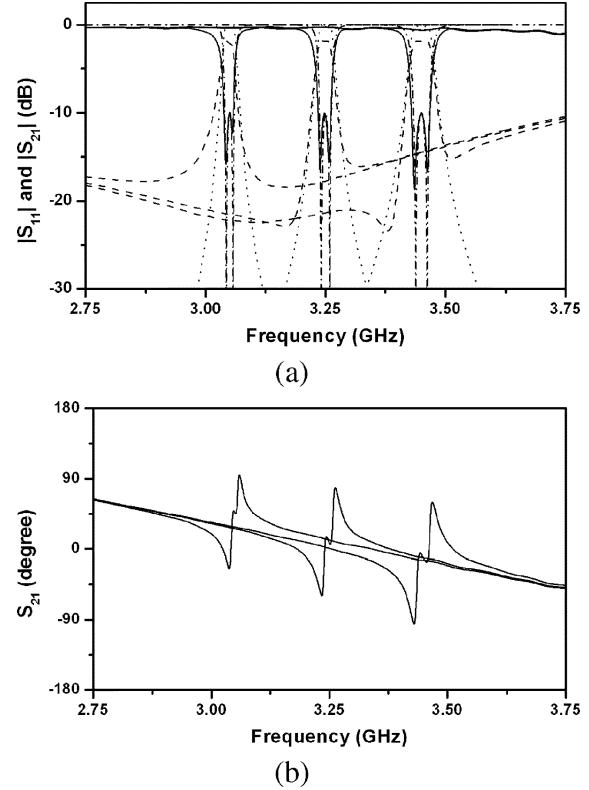
Fig. 4. Measured frequency response of the fabricated bandstop filter. The filter is tuned to exhibit Chebyshev bandstop responses with 10 dB stopband rejection at three different center frequencies: (a)  $|S_{11}|$  measurement (— —),  $|S_{21}|$  measurement (— —),  $|S_{11}|$  synthesis (· · ·),  $|S_{21}|$  synthesis (— — —), (b)  $S_{21}$  (degree) measurement.
