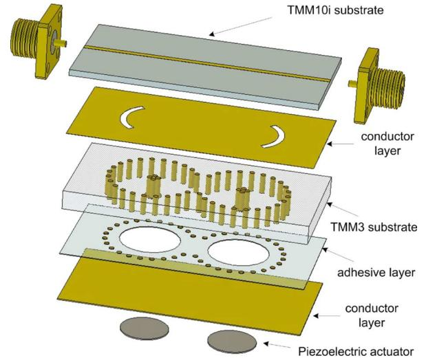
Fig. 2. Proposed bandstop filter with two substrated-integrated evanescent-mode cavity resonators.
