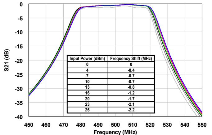
**Figure 5 - Shift in filter response with power level.**
