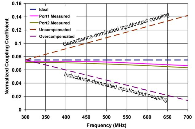
Figure 3 - Measured input/output coupling coefficients of frequency-tailored coupling networks.
