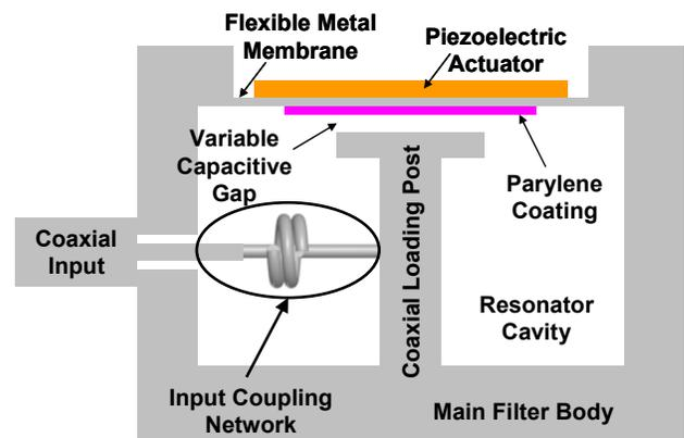
Figure 1 - Cross-section view of a capacitively-loaded cavity with a piezo actuator for mechanical deflection.
