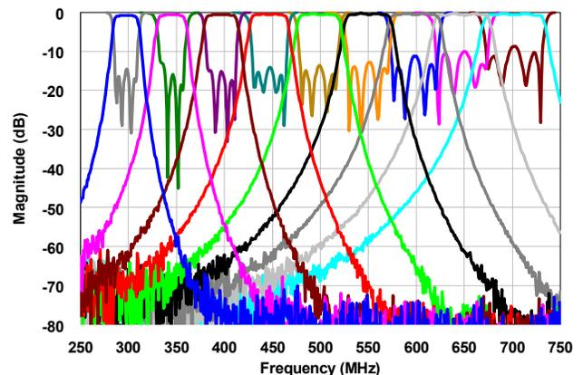
Figure 4 - Multi-pole tunable UHF filter response
