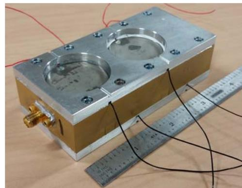
Figure 2 - Four-pole tunable filter at UHF frequencies.
