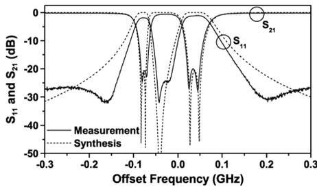
Fig. 7. Synthesized and measured results of asymmetric equi-ripple response.
