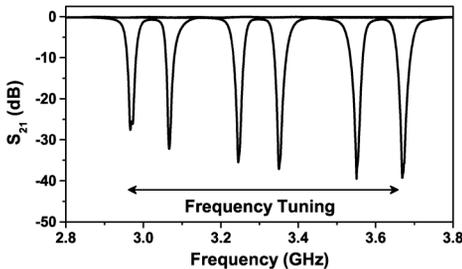
Fig. 8. Measured results with different center frequencies.
