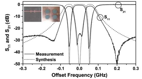
Fig. 4. Synthesized and measured results of symmetric Butterworth response.
