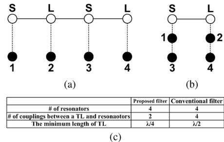
Fig. 1. Routing diagram of the 2nd-order dual-stopband filter (a) conventional dual-stopband filter (b) proposed dual-stopband filter (c) comparison between proposed topology and conventional one.
