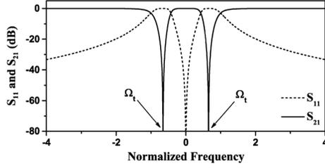
Fig. 2. Theoretical results of a symmetric Butterworth response in the normalized frequency domain.
