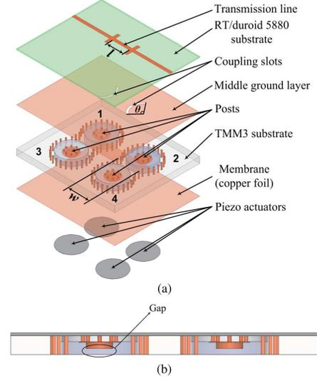
Fig. 3. 3D-view of the designed filter (a) layer-by-layer structure ( $l = 9$  mm,  $w = 11.2$  mm,  $\theta = 104^\circ$ ) (b) side-view. The gap between the post and the membrane is exaggerated and some of via-holes are not shown for the reader's convenience. The resonant frequency of each resonator can be controlled by adjusting this gap by means of a piezo actuator whose deflection range limits the tuning range of each resonator.
