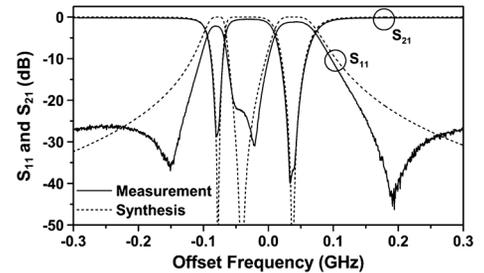
Fig. 6. Synthesized and measured results of asymmetric Butterworth response.
