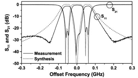
Fig. 5. Synthesized and measured results of symmetric equi-ripple response.
