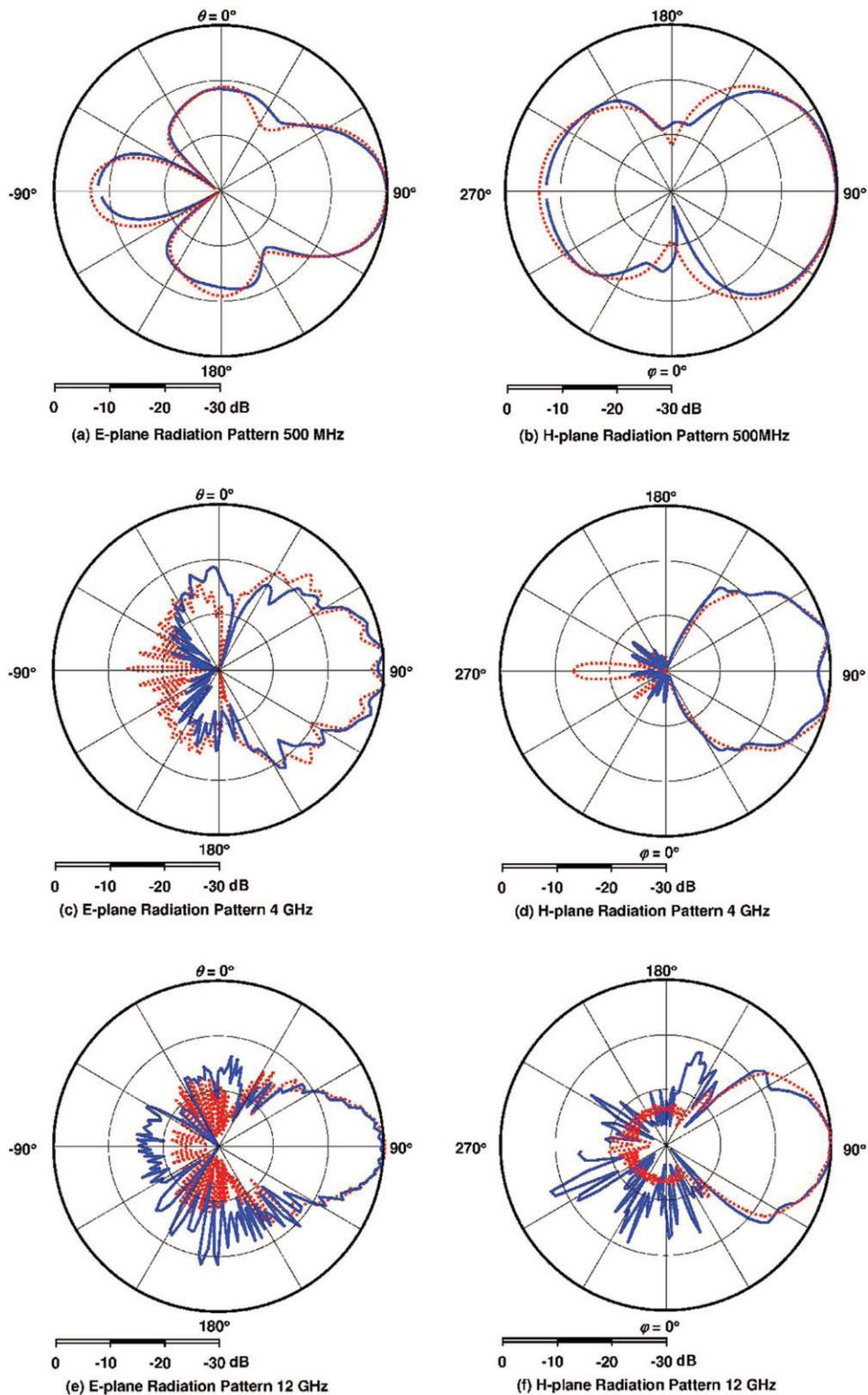
**Figure 4** *E* and *H* plane radiation patterns. (a) and (b): 500 MHz; (c) and (d): 4 GHz; (e) and (f): 12 GHz. \_\_\_\_ Measured . . . . . Calculated. [Color figure can be viewed in the online issue, which is available at [www.interscience.wiley.com](http://www.interscience.wiley.com)]
