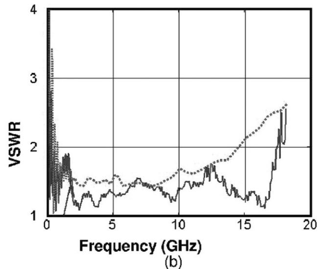
**Figure 3** Response of VSWR versus frequency. (a) Expanded lower frequency region, and (b) VSWR through 18 GHz. — Measured . . . . . Calculated. [Color figure can be viewed in the online issue, which is available at [www.interscience.wiley.com](http://www.interscience.wiley.com)]
