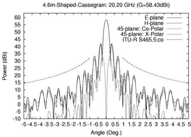
Figure 6 Radiation pattern of the antenna at 20.20 GHz
