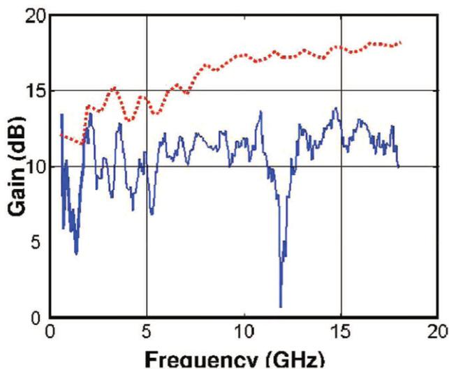
**Figure 5** Response of Gain versus frequency. \_\_\_\_ Measured ..... Calculated. [Color figure can be viewed in the online issue, which is available at [www.interscience.wiley.com](http://www.interscience.wiley.com)]
