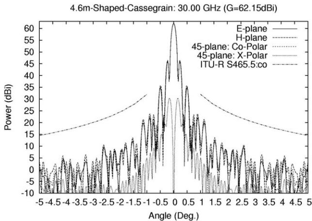
Figure 7 Radiation pattern of the antenna at 30.00 GHz
