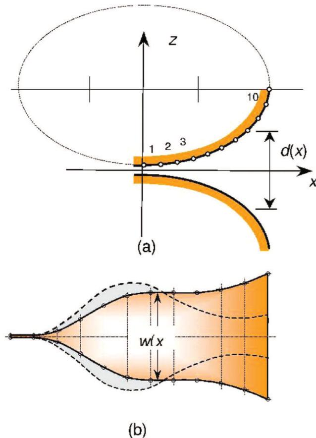
**Figure 1** (a) Profile of the elliptic horn, side view; (b) plate profile with parallel plate impedance equation compared to stripline equation (dashed line). [Color figure can be viewed in the online issue, which is available at [www.interscience.wiley.com](http://www.interscience.wiley.com)]
