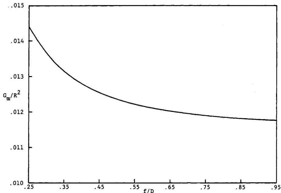
Fig. 9. Maximum gain/tolerance ratio squared versus reflector  $f/D$ .
