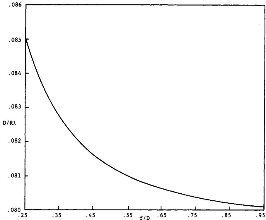
Fig. 8. Reflector diameter/tolerance ratio versus  $f/D$ .
