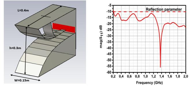
Fig. 4. K Antenna and reflection coefficient magnitude
