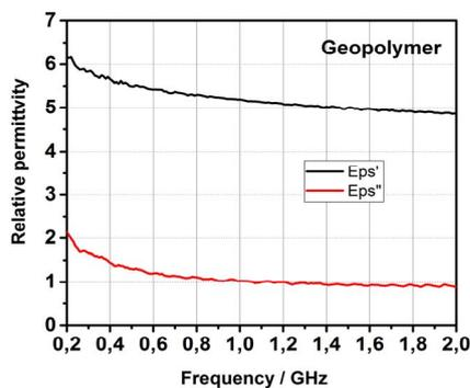
Fig. 10. Real part ( $\epsilon'_{ps}$ ) and Imaginary part ( $\epsilon''_{ps}$ ) of relative permittivity - Geopolymer
