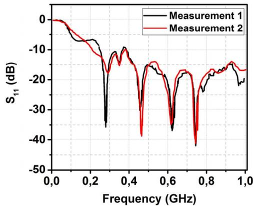
Fig. 9. Measured adaptation parameter; influence of soil humidity
