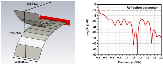
Fig. 3. Unbalanced Antenna and reflection coefficient magnitude
