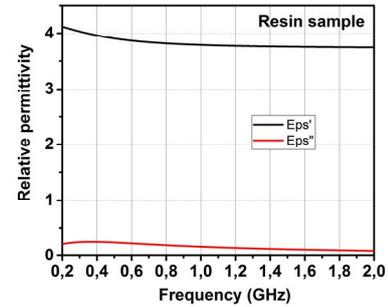
Fig. 7. Real part ( $Eps'$ ) and Imaginary part ( $Eps''$ ) of relative permittivity - resin sample
