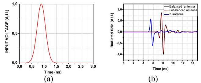
Fig. 5. Dispersion analysis: (a) Input voltage (b) Radiated field of the antennas
