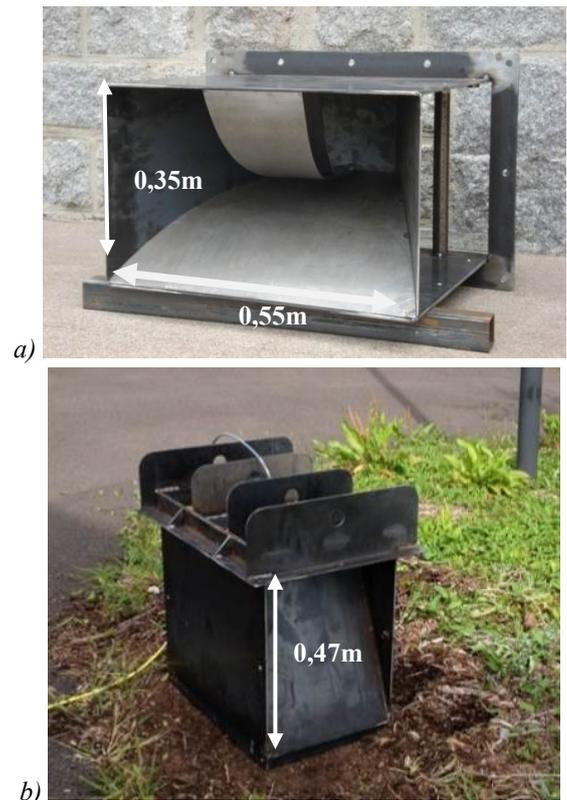
Fig. 8. KHORN Antenna: a) Metallic structure, b) Antenna, filled using the resin, in contact with soil
