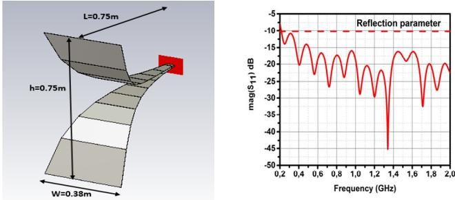
Fig. 2. Balanced Antenna and reflection coefficient magnitude
