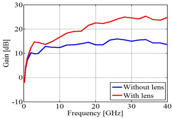
Fig. 8. Miniaturized combined antenna gain in terms of frequency with and without lens
