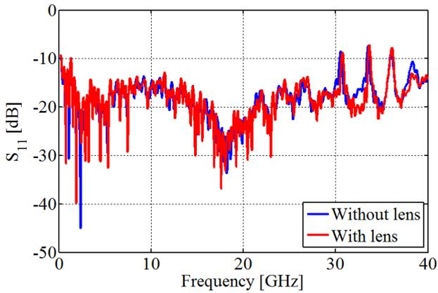
Fig. 6. Simulated return-loss of the proposed miniaturized combined antenna with and without lens
