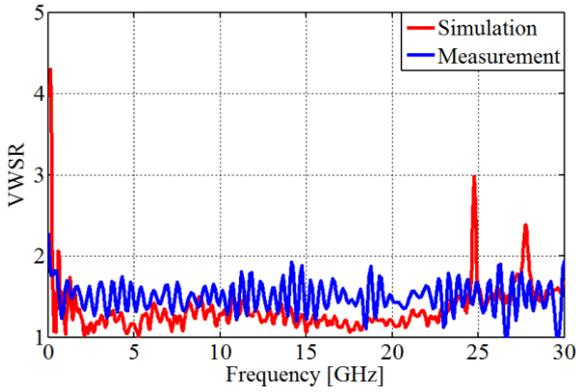
Fig. 2. VSWR resulted from simulation and fabrication
