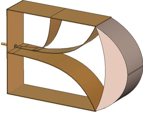
Fig. 5. Miniaturized combined antenna with lens
