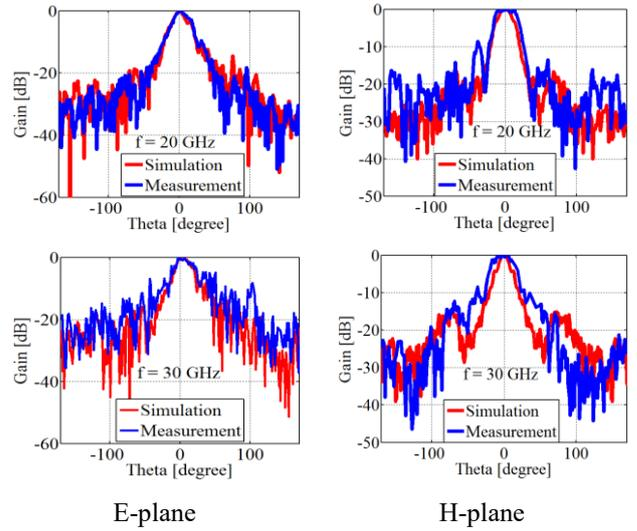
Fig. 3. Antenna pattern resulted from simulation and fabrication.
