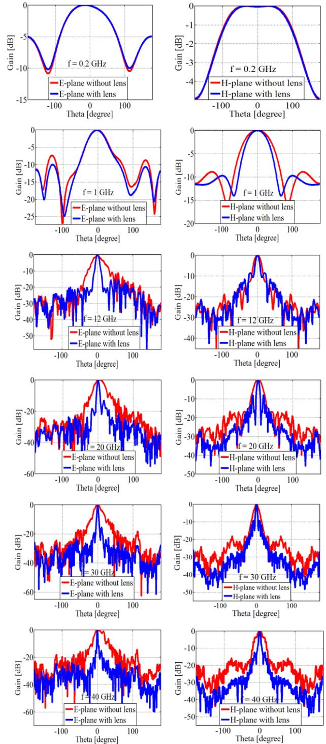
Fig. 7. Simulated radiation patterns of the proposed miniaturized antenna with and without lens at different frequencies
