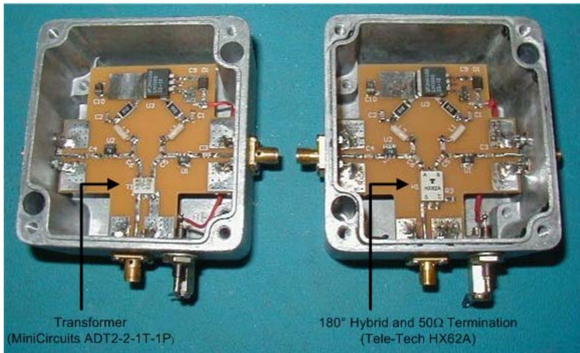
**Figure 2 – Single Polarization Test Baluns**
