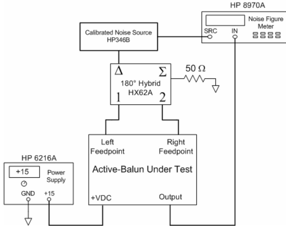
**Figure 13 - Noise Figure Measurement Setup**
