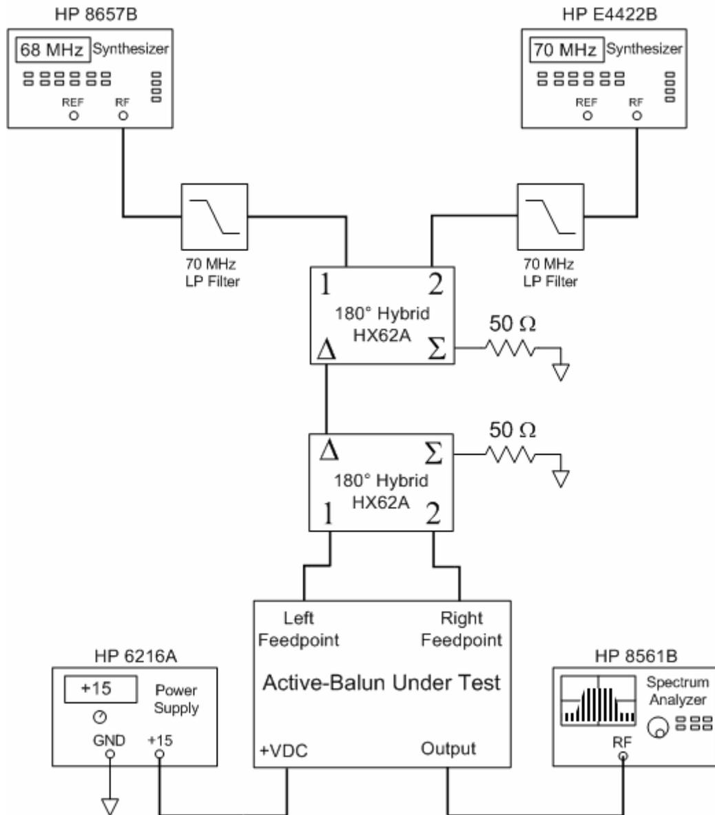
Figure 12 - IMD Measurement Setup
