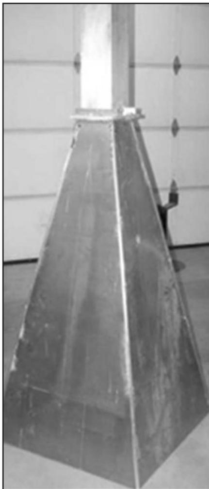
Figure 5. CP horn antenna using all-aluminum construction.
