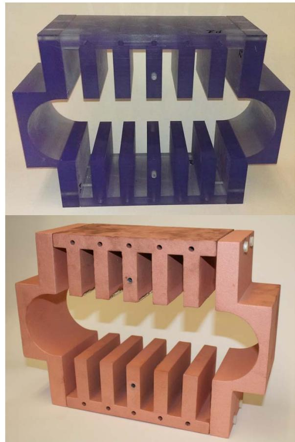
**Figure 1.** a) (Top) 3-D printed plastic anode prior to metallization. b) (Bottom) The same anode after thermal spraying.
