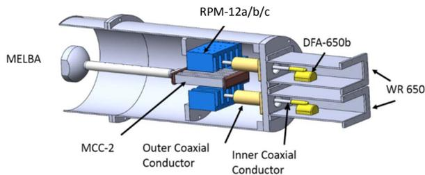
**Figure 2.** Experimental configuration for RPM-12a/b/c experiments. Anode region shown in blue, directional couplers and loads not shown.
