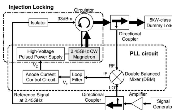
**Figure 1.** A schematic diagram of a pulse-driven phase-controlled magnetron
