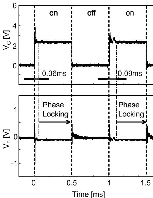
**Figure 2.** Experimental results of the pulse-driven phase-controlled magnetron (upper: control voltage of the power supply  $V_C$ , lower: mixer output  $V_F$ )
