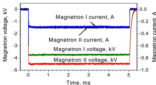
Figure 2: Traces of currents and voltages of magnetrons operating simultaneously in injection-locked mode.
