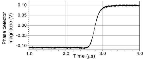
FIG. 8: Response of the frequency-locked 2-cascade magnetron on the 180 degrees phase flip measured at ratio of the output power to locking power  $\approx 27$  dB; the phase detector calibration is  $\approx 0.8$  degrees/mV.
