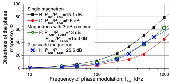
Figure 13: Performance of the injection-locked magnetrons vs. frequency of the phase modulation,  $f_{PM}$ , as controlled by the phase-modulated signal.
