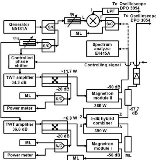
Figure 9: Setup with the injection-locked magnetrons for test of the power control by power combining.
