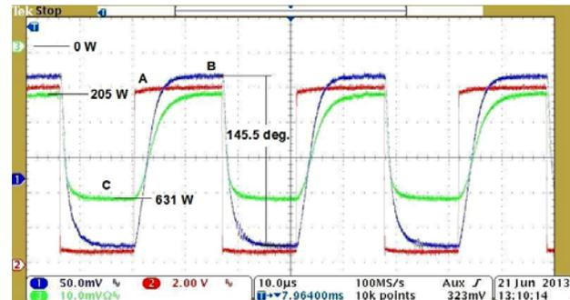
Figure 11: Trace A is shape of the voltage, controlling the phase shifter JSPHS-2484, trace B is the magnetron II phase response on the shifter fast control, trace C shows variation of the power measured by the calibrated detector at the port “ $\Sigma$ ” of the 3 dB hybrid.
