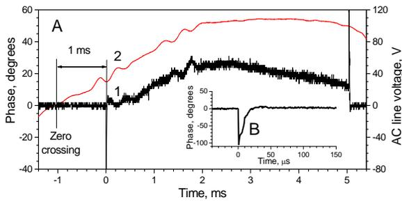
Figure 12: A- phase variations of the combined in power injection-locked magnetrons; B- zoomed in time trace 1.
