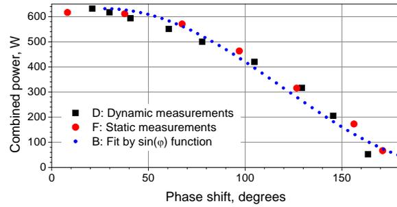
Figure 10: Control of combined power of the injection-locked magnetrons by the phase difference. Dots F and D present power variation at the combiner port “ $\Sigma$ ”, measured in static and dynamic regimes, respectively. Dots B show fit of the plots D and F by  $\sin(\varphi)$  function.
