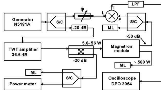
Figure 3: Experimental setup to test and study operation of magnetrons in injection-locked mode. S/C is a 3-dB splitter/combiner; ML is a matched load.
