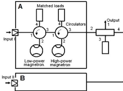
Figure 1: Block-diagram of the high-power magnetron RF source rapidly controlled in phase and power.
