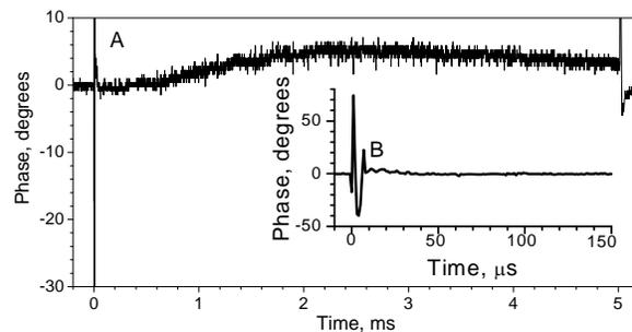
Figure 4: A- phase variation of the injection-locked CW magnetron operating at locking power of -9.6 dB, and a pulse duration of 5 ms. Inset B shows the phase variation zoomed in time.
