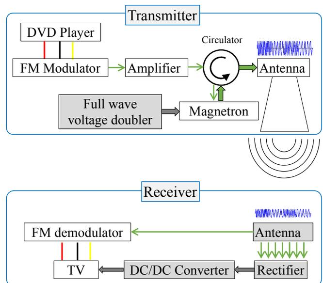
Fig. 1 Wirelessly-powered TV system diagram.
