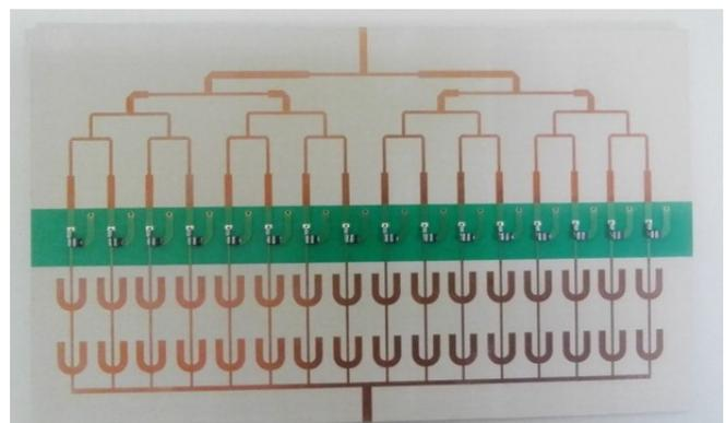
Fig. 2 Photo of a 2.45GHz rectifier circuit board
