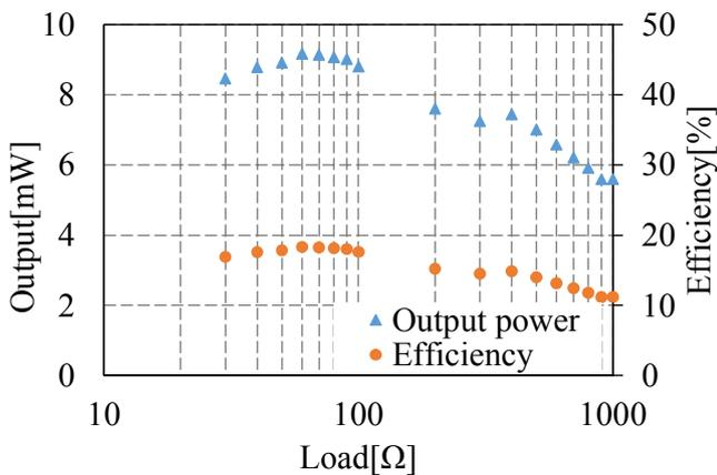
Fig. 3 Rectifier efficiency of the rectifier circuit with different load(input 50mW).
