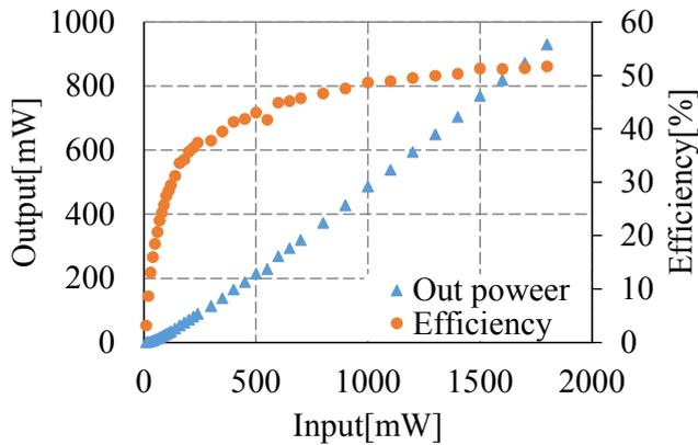
Fig. 4 Rectifier efficiency of the rectifier circuit with different input power(load: 60 $\Omega$ )
