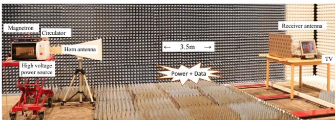
Fig. 5 Photo of the wirelessly-powered TV.
