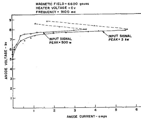
Fig. 10—Anode voltage vs anode current.
