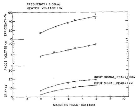
Fig. 8—Characteristics vs magnetic field.
