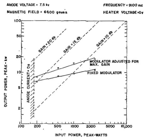
Fig. 6—Drive characteristics.
