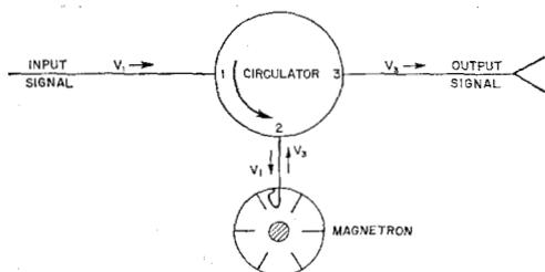
Fig. 1—Schematic diagram of the amplifier circuit.
