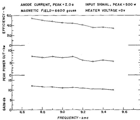
Fig. 5—Characteristics vs frequency. Constant anode current.
