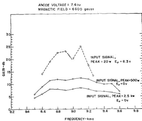
Fig. 7—Maximum gain vs frequency.
