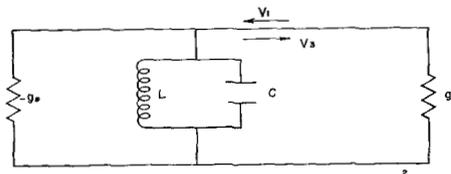
Fig. 2—Equivalent circuit of magnetron arm.
