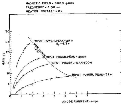
Fig. 9—Gain vs anode current.
