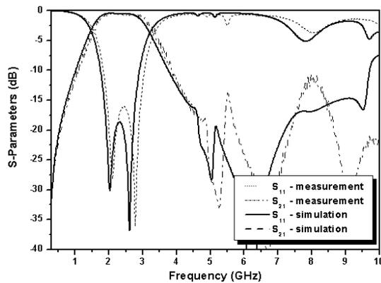
Fig.7. Simulated and measured frequency response of the proposed ring-type bandpass filter.
