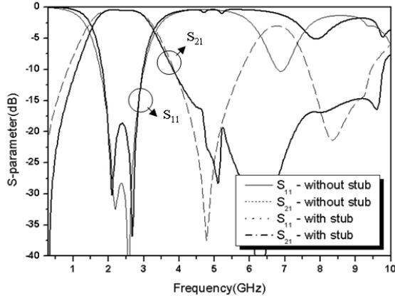
Fig. 5. Simulated frequency response of the proposed ring-type bandpass filters with/without the internal open-circuited stubs.
