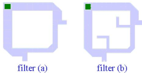
Fig. 4. Schematic diagrams of the proposed ring-type bandpass filters (a) without the internal open-circuited stubs and (b) with the internal open-circuited stubs.
