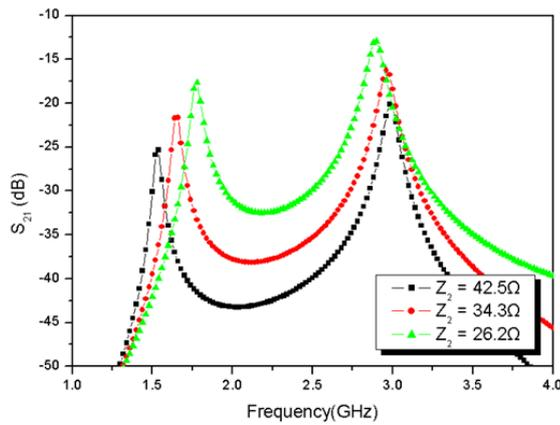
Fig. 3. Frequency response of  $S_{21}$  under varied impedance of short-circuited stubs ( $Z_2$ ).
