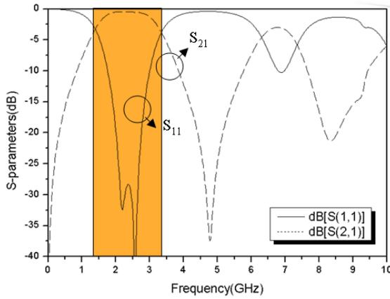
Fig.2. Simulated frequency response of the proposed ring-type BPF.
