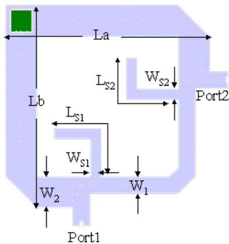
Fig. 6. Configuration of the proposed ring-type bandpass filter.
