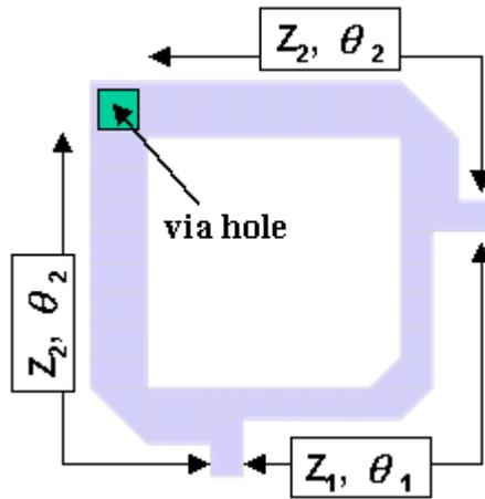
Fig. 1. Schematic diagrams of proposed ring-type bandpass filter.
