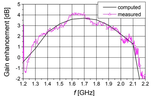
Figure 6. Computed and measured enhancement of helix gain [1]
