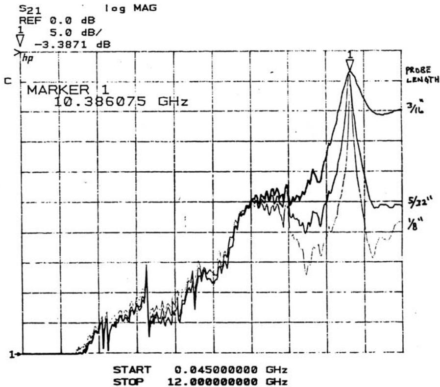
Figure 14. Measured response of 1/2" pipe-cap filter
