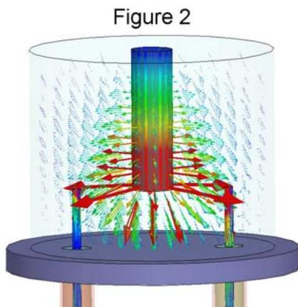
tuning screw acts as the coax center conductor, with a radial electric field around it; the field intensity increases toward the open end of the screw. The resonant frequency is determined by the inserted length of the screw; Figure 3 shows that the same screw length produces the same resonant frequency in three different sizes of pipe caps. The other dimensions do not affect the frequency, as they would if a waveguide cavity mode were involved.
