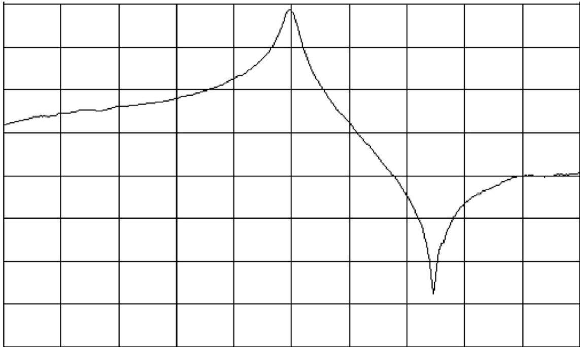
**Figure 4 - Over coupled filter response. Center frequency 738 MHz, top reference line 0 DBm, span 100/MHz division horizontal, 10-DB/div vertical**
