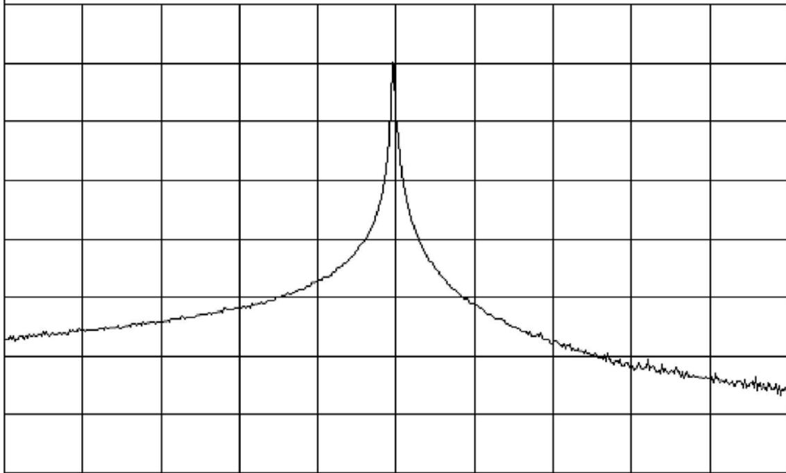
**Figure 5 - Response after adjusting coupling loops but loops moved during soldering as insertion loss increased from 6 to 9 DB. 3-DB bandwidth is 1.3 MHz. Loops were adjustable for less insertion loss and wider bandwidth. Center frequency 738 MHz, top reference line 0 DBm, span 50 MHz/division horizontal, 10-DB/division vertical.**
