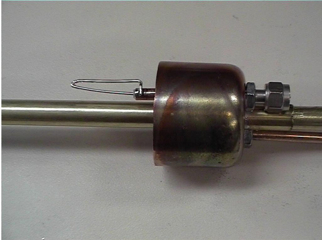
**Figure 2 - Coupling loop detail**
