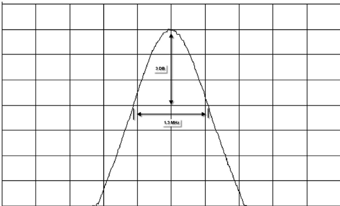
**Figure 6 - Filter 3-DB bandwidth. Center frequency 738 MHz, span 500 KHz/div horizontal, 1-DB/div vertical**
