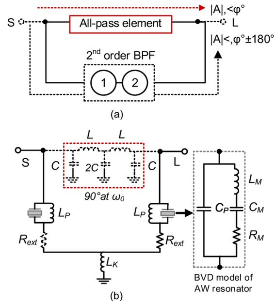
Fig. 1. (a) Generic block diagram of a two-path ABSF [2]. (b) Schematic circuit of a narrowband ABSF that makes use of high- $Q$  one-port SAW resonators—represented by the Butterworth Van-Dyke circuit model in [11]—and lumped-element impedance inverters.
