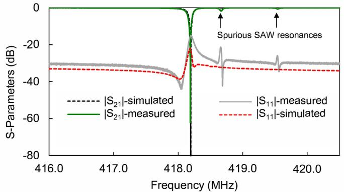
Fig. 4. Simulated and measured responses of the manufactured prototype in Fig. 3.
