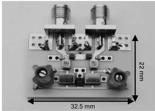
Fig. 3. Manufactured prototype. The utilized components for 0.02% 3-dB FBW are:  $C$ : Johanson Tech. 250R05L2R7CV4T,  $2C$ : Johanson Tech. 251R14S5R6CV4T,  $R_{ext}$ : Bourns 3314J-1-200E,  $L_K$ : Coilcraft 0805HT-6N8,  $L$ : 0806SQ-12N, SAW resonator: Abracon ASR418S2— $L_A=119.67 \mu\text{m}$ ,  $C_M=1.211 \text{ fF}$ ,  $R_M=22.2 \text{ Ohm}$ ,  $C_P=1.59 \text{ pF}$  are its BVD equivalent parameters that have been extracted from the measured response of a single SAW resonator prototype).
