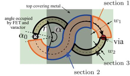
**Fig. 9** Division of figure of eight resonator for design.
