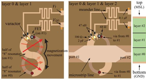
**Fig. 7** Tunable microwave isolator using figure of eight resonator, consisting of varactor inserted figure of eight resonator over two layers. The ring is organised in two layers, and as a consequence one layer is added to Fig. 4.
