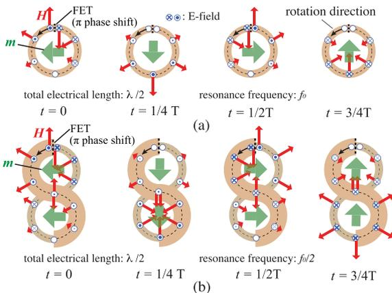
**Fig. 8** Vectorial fields comparison of magnetic field in FET inserted (a) simple ring resonator and (b) figure of eight ring resonator for one harmonic period, assuming 180° phase shift FET is inserted on the top of figures.
