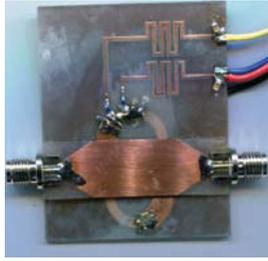
Fig. 11 Picture of prototype isolator corresponds to Fig. 7.
