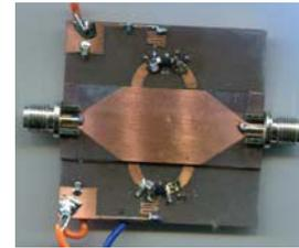
Fig. 5 Picture of prototype isolator corresponds to Fig. 4.
