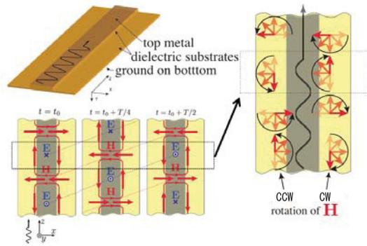
Fig. 2 General quasi-TEM wave propagation in microstrip line.
