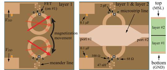
Fig. 4 Isolator configuration based on the principle in Fig. 3.
