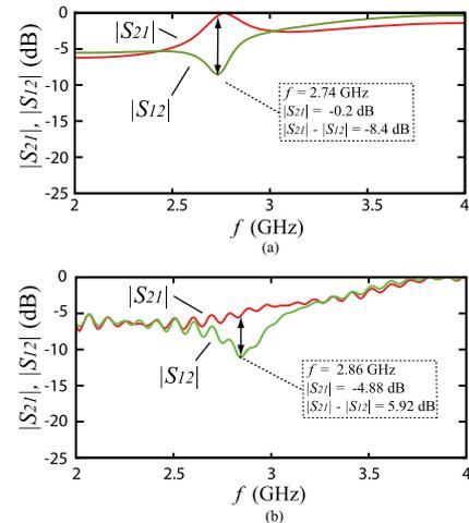
Fig. 6 Transmission characteristics of the isolator in Fig. 4. (a) Simulation results. (b) Measured value.
