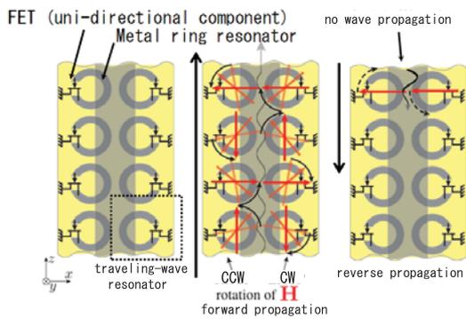
Fig. 3 Principle of isolator operation using MNM.
