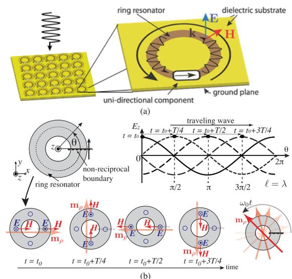
**Fig. 1** Principle of Magnet-less Non-reciprocal Metamaterial (MNM). (a) Unit-cell configuration consisting of uni-directional component inserted metal ring resonator on substrate. (b) Vectorial field explanation.
