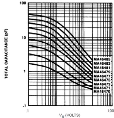
**Fig. 10** Varactor diode (MA46470) response for reverse voltage in [7].
