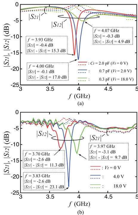
Fig. 12 Transmission characteristics of the prototype isolator in Fig. 7. (a) Simulation results. (b) Measured value obtained by the device in Fig. 11.
