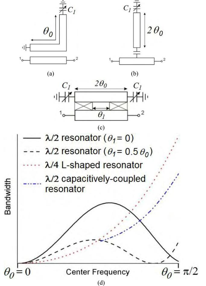
Fig. 4. Diagrams of bandstop filters with capacitively-tuned (a) edge-coupled L-shaped  $\lambda/4$ , (b) capacitively-coupled  $\lambda/2$ , and (c) edge-coupled  $\lambda/2$  resonators, and (d) a plot of the simulated bandwidth versus tuned center frequency for each filter.  $2\theta_0$  is the electrical length of the  $\lambda/2$  resonators at the tuned center frequency and  $\theta_l$  is the centered portion of the edge-coupled resonator decoupled from the through line.
