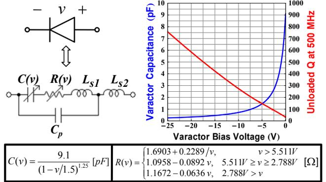
Fig. 5. Model of the reverse-biased Metelics MGV-125-26-0805 GaAs hyperabrupt varactor diode, with  $L_{s1}=0.4nH$ ,  $L_{s2}=0.86nH$ , and  $C_p=0.07pF$ .
