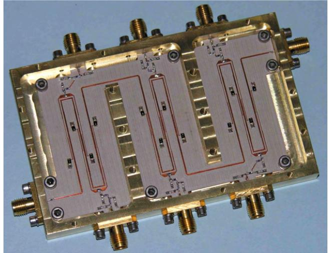
Fig. 6. (a) Annotated layout of a single-stage tunable absorptive notch filter and (b) photo of a corresponding three-stage filter in a 101.6 x 63.5 x 8.9 mm brass enclosure with SMA connectors.
