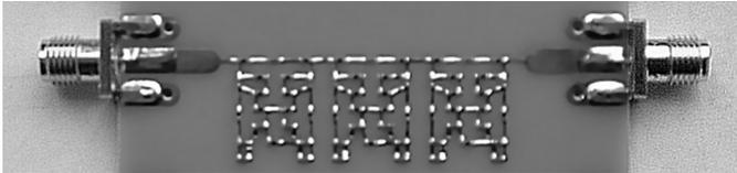
Fig. 14. Photograph of the reflectionless band-pass filter prototype.
