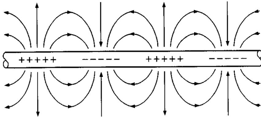
**Figure 2.2** RF charge (+ and -) and electric field patterns (solid lines) for a single-wire transmission line above a ground plane. Reprinted with permission from Principles of Traveling Wave Tubes, by A. S. Gilmour, Jr., Artech House Publishers, Norwood, MA, USA. [www.artechhouse.com](http://www.artechhouse.com) [Gilmour, 1994]
