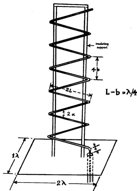
**Figure 2.8.** Diagram showing the zig-zag antenna with feeding arrangement [Sengupta, 1958]
