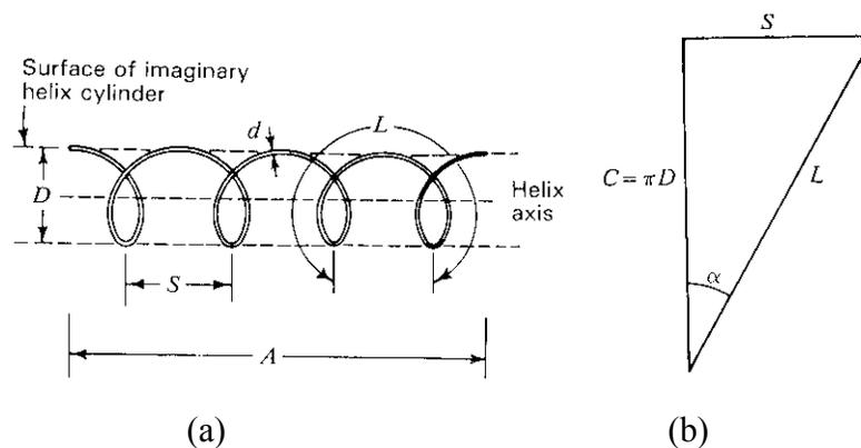
**Figure 2.4** Basic helix geometry defining diameter ( $D$ ), turn-to-turn spacing ( $S$ ), axial length ( $A$ ), circumference ( $C$ ), turn length ( $L$ ), and pitch angle ( $\alpha$ ). In (b) the relationships between  $S$ ,  $C$ ,  $D$ ,  $L$  and  $\alpha$  are shown for a single turn that has been stretched out flat. [Kraus, 1988]
