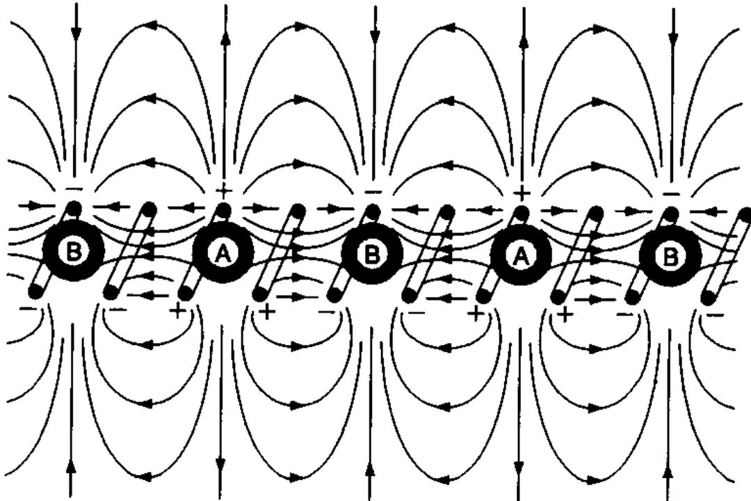
**Figure 2.3.** RF charge and electric field patterns for a helix. Reprinted with permission from *Principles of Traveling Wave Tubes*, by A. S. Gilmour, Jr., Artech House Publishers, Norwood, MA, USA. [www.artechhouse.com](http://www.artechhouse.com) [Gilmour, 1994]
