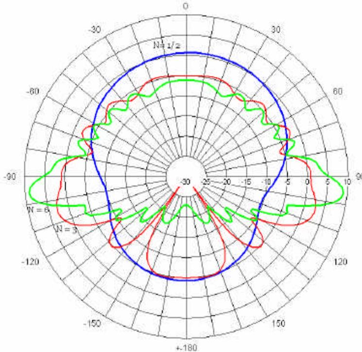
**Figure 2.6** NEC simulated radiation patterns of quadrifilar helices with  $N = 1/2$ ,  $N = 3$ , and  $N = 6$  turns showing how the main lobe of the pattern moves from on-axis to broadside of the quadrifilar as the number of turns is increased. The helix axis is aligned with  $\theta = 0^\circ$ , the same orientation as in Figure 2.5.
