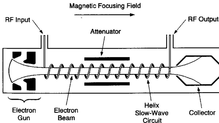
**Figure 2.1** Basic helix traveling wave tube amplifier. Reprinted with permission from Principles of Traveling Wave Tubes, by A. S. Gilmour, Jr., Artech House Publishers, Norwood, MA, USA. [www.artechhouse.com](http://www.artechhouse.com) [Gilmour, 1994]
