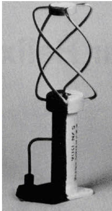
**Figure 2.5.** Typical quadrifilar helix or volute antenna [Maxwell, 1990]
