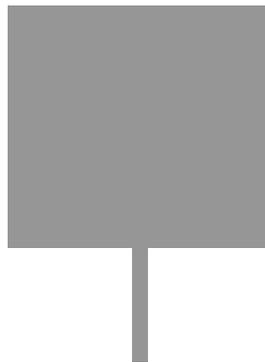
*Figure 12: Microstrip line fed patch antenna*
