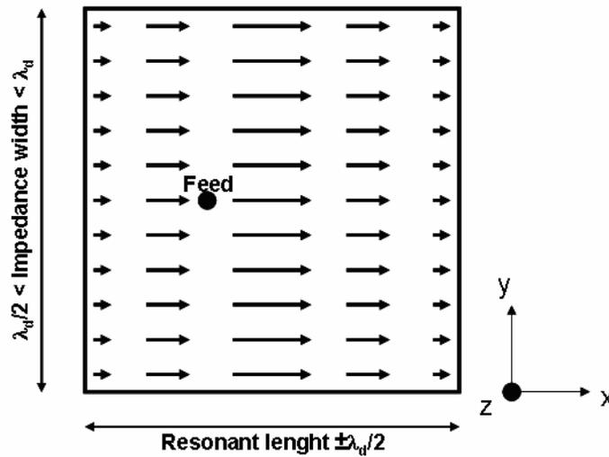
*Figure 2: Current distribution on the patch surface*
