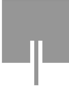
**Figure 13:** *Inset microstrip line fed patch antenna*
