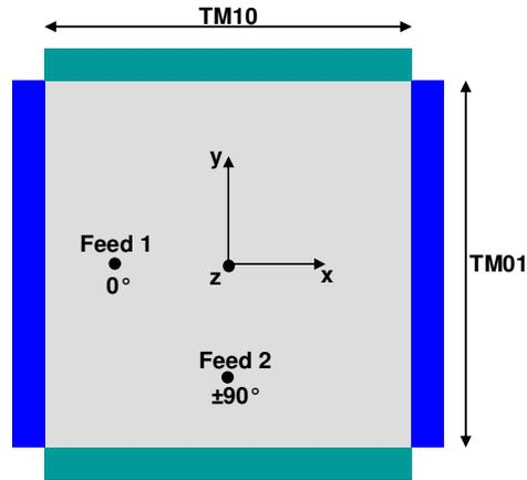
**Figure 5:** The nearly square mechanism for circular polarization
