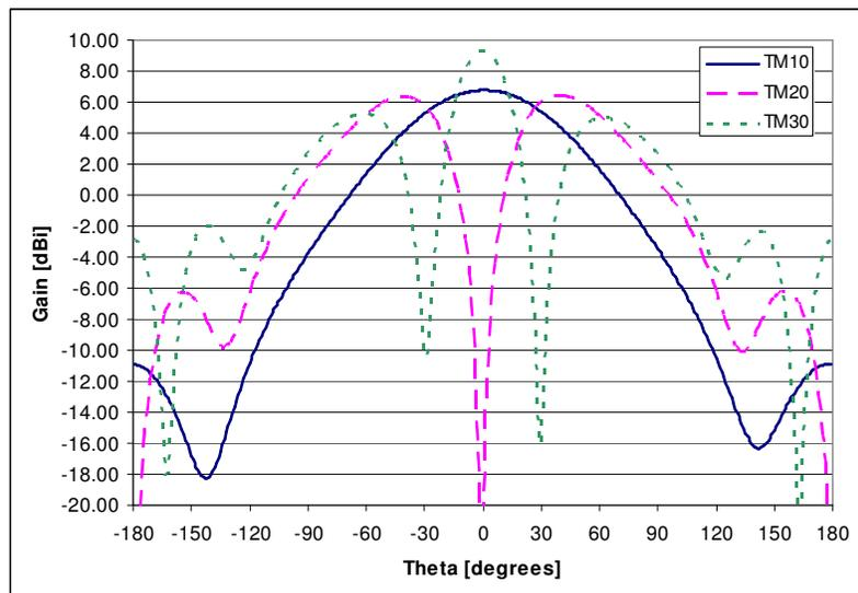
*Figure 23: Radiation patterns of higher rectangular patch modes*
