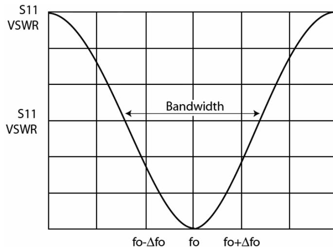
**Figure 10:** Impedance bandwidth definition
