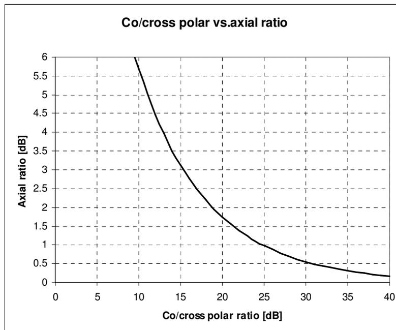
*Figure 9: Co/cross polar ratio versus axial ratio*
