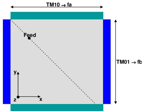
*Figure 7: Nearly square patch fed on the diagonal*
