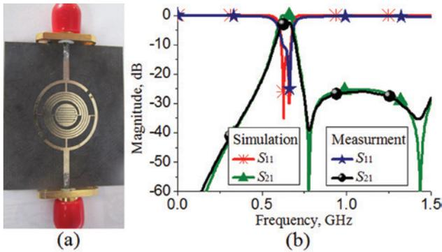
Fig. 4: BPF 2: (a) picture, (b) results.
