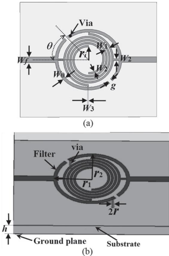
Fig. 1: Configuration of BPF 1: (a) top view, (b) 3D view.
