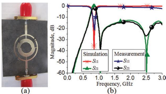
Fig. 2: BPF 1: (a) picture, (b) results.
