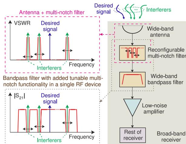
Fig. 1. Block diagram and operational principle of a broad-band receiver with incorporated reconfigurable-multi-notch RF filtering functionality for dynamic multi-interference mitigation ( $|S_{21}|$ : power transmission response; VSWR: voltage standing wave ratio). Note that the devised reconfigurable RF filtering solution incorporates both functionalities at the same filter volume.
