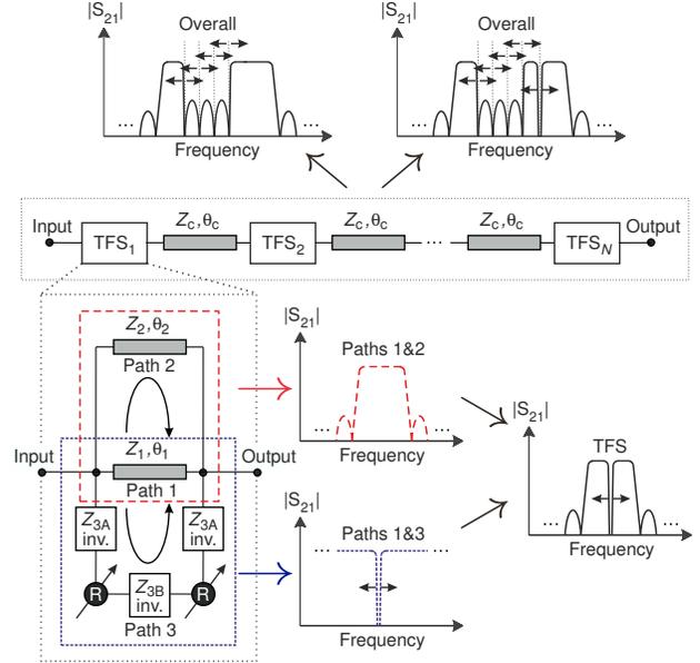
Fig. 2. Circuit detail and operational principles of the proposed multi-stage wide-band bandpass filter with embedded tunable in-band notches (“TFS”: transversal filtering section; “R”: resonator;  $Z$ : characteristic impedance;  $\theta$ : electrical length).
