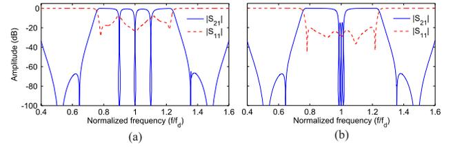
Fig. 3. Theoretical power transmission ( $|S_{21}|$ ) and reflection ( $|S_{11}|$ ) responses for two different states of a three-stage design based on the RF filter concept in Fig. 2. (a) Response with spectrally-separated in-band notches. (b) Response with the three in-band notches shaping a three-transmission-zero wider stopband.
