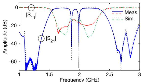
Fig. 5. Simulated and measured power transmission ( $|S_{21}|$ ) and reflection ( $|S_{11}|$ ) of the manufactured prototype for one state.
