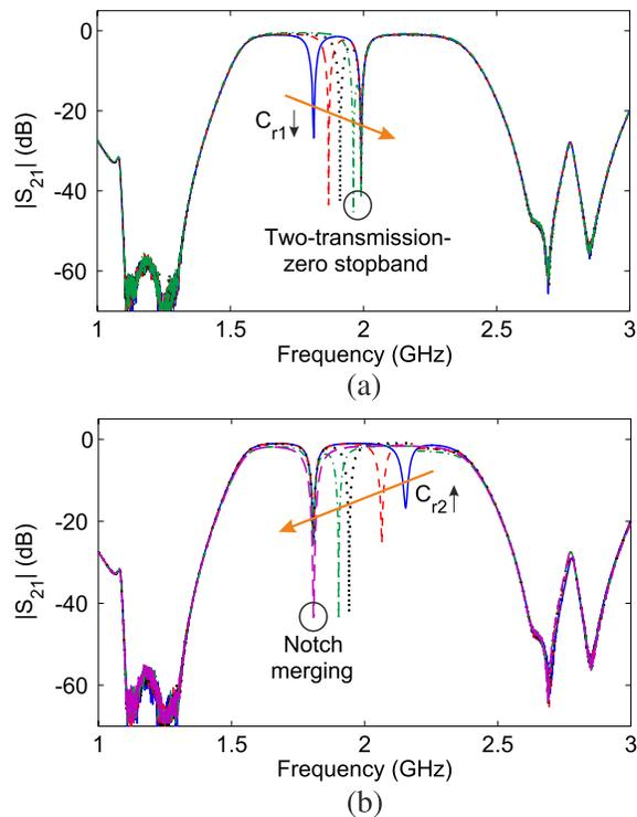
Fig. 6. Measured reconfiguration capabilities of the manufactured prototype in terms of power transmission response ( $|S_{21}|$ ). (a) Frequency tuning of the lower in-band notch and shaping of a two-transmission-zero stopband when it comes to a close proximity to the upper in-band notch. (b) Frequency tuning of the upper in-band notch and spectral merging with the lower one.
