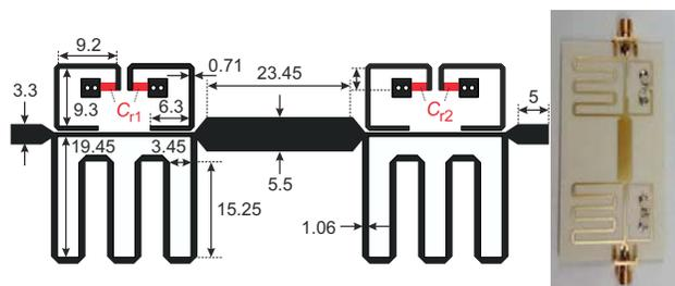
Fig. 4. Layout and photograph of the manufactured prototype (dimensions, in mm, are indicated).
