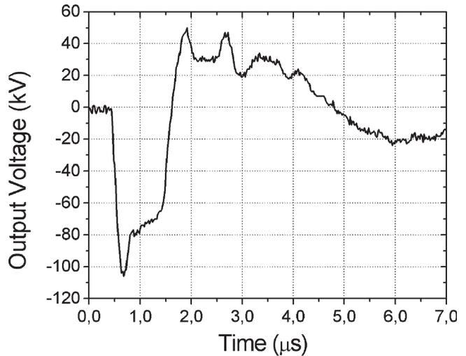
Fig. 3. Maximum peak voltage obtained of 100 kV.
