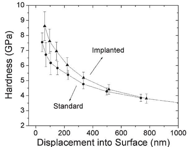
Fig. 7. Hardness profiles obtained for the implanted SS304 and standard (nontreated) samples.
