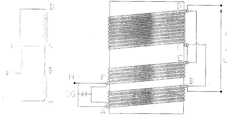
Figure 3. Winding arrangement and layout of double-Blumlein generator.
