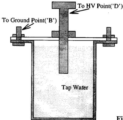
Figure 8. Schematic of tap water load.
