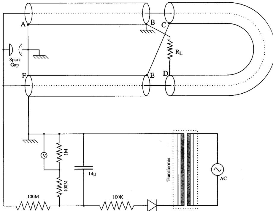
**Figure 2.** Schematic of constructed double-Blumlein pulse power supply.
