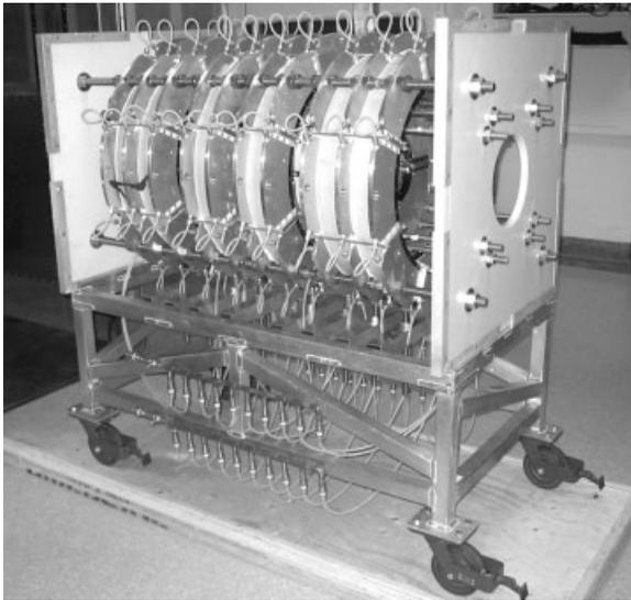
**Figure 9** A photograph of two concentric magnets and the support structure. The system was built and cooled using the construction technique described in this article.
