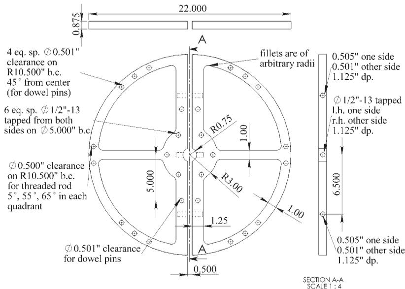
**Figure 2** A schematic of the inner portion of the aluminum bobbin. Several plates can be stacked together to form a bobbin of any desired width. The two halves of the bobbin are connected by a left-hand right-hand threaded stud. All dimensions are given in inches. Eq. sp. = equally spaced; b.c. = bolt circle; l.h. = left-hand; r.h. = right-hand; dp. = deep.
