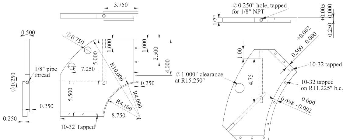
**Figure 5** A schematic of a single section of a (left) one-piece four-section cooling plate with rim and (right) an eight-section cooling plate with detachable rim. All dimensions are given in inches. b.c. = bolt circle; NPT = National Pipe Thread.
