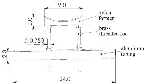
**Figure 7** A schematic of a nylon brace used to support the mass of a coil. The nylon brace is adjustable in height. All dimensions are given in inches.
