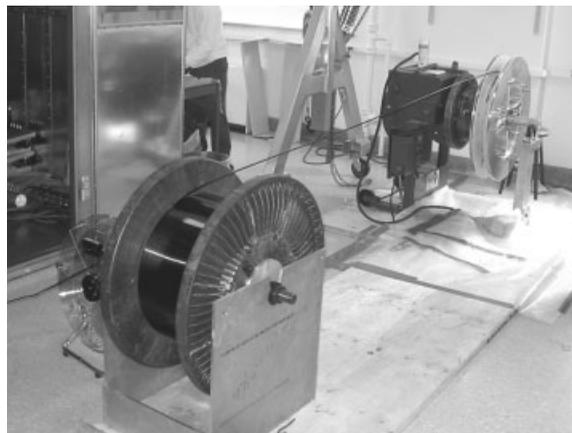
**Figure 1** The system employed to wind the magnet coils. The wire is drawn off a tensioned spool (left) onto a bobbin (right), which is rotated by a cylindrical welding positioner (right).
