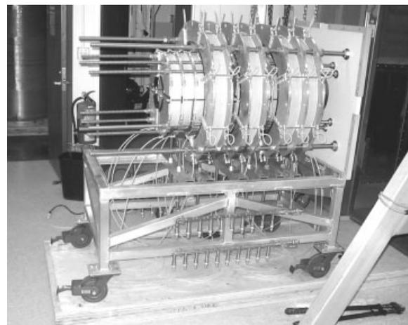
**Figure 6** A photograph of a partially assembled field-cycled MRI system. Coils were successively moved into position by a chain-fall gantry. Threaded rods are attached to 1-inch-thick nylon plates at each end, off of which cooling plates and coils are suspended. The coils are supported by adjustable-height nylon braces. The outer homogeneous magnet is the readout magnet, and the inner solenoid is the polarizing magnet (12).
