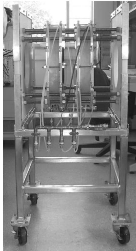
**Figure 8** A photograph of a thick Helmholtz pair built and cooled using the construction technique described in this article. The system has a 21-cm inner diameter and weighs approximately 75 kg. The coil pair produces a field efficiency of 1.3 mT/A.
