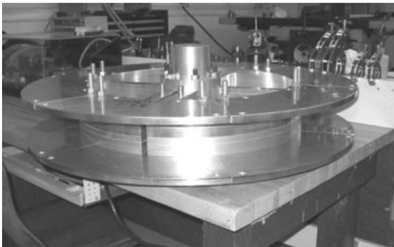
**Figure 3** A photograph of the entire collapsible bobbin. The removable side plates sandwich the collapsible inner cylinder.
