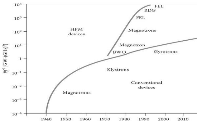
Fig. 3. Growth of microwave devices in terms of the figure of merit  $Pf^2$ , with identify the year when the plotted value of  $Pf^2$  was first achieved [1]
