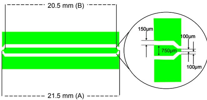
Figure 2. Layout of Ink-Jet Printed CPW Line
