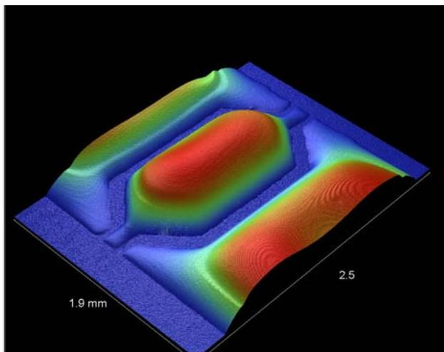
Figure 5. 3D image of CPW obtained with a Veeco white light interferometer.
