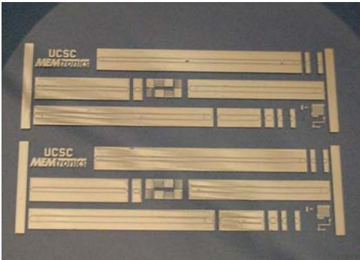
Figure 3. Photograph of Printed CPW Lines on Glass Substrate
