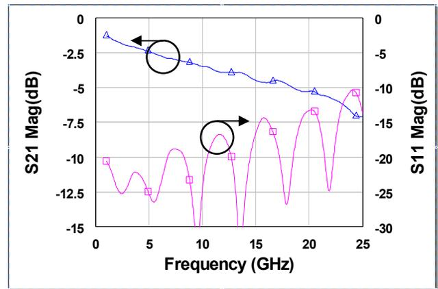
Figure 4. S11 and S21 of Printed CPW Line
