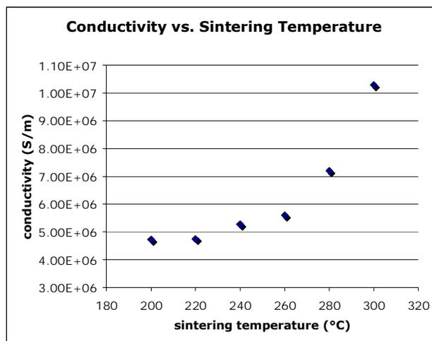
Figure 1. Conductivity vs. sintering temperature for Cabot silver nano-particles ink jetted with a Dimatix printer onto a surface treated glass substrate.
