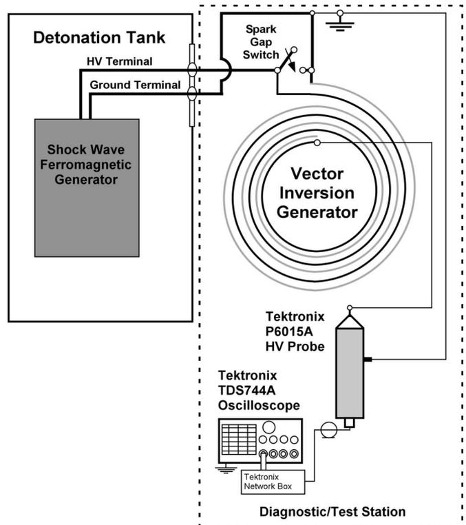
Fig. 3. Schematic diagram of the experimental setup used to test the completely explosive FMG–VIG system.
