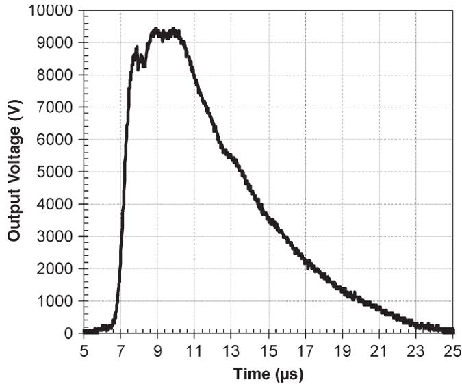
Fig. 6. Waveform of the pulsed EMF produced by an FMG (257-turn pulse-generating coil). Open-circuit operation.
