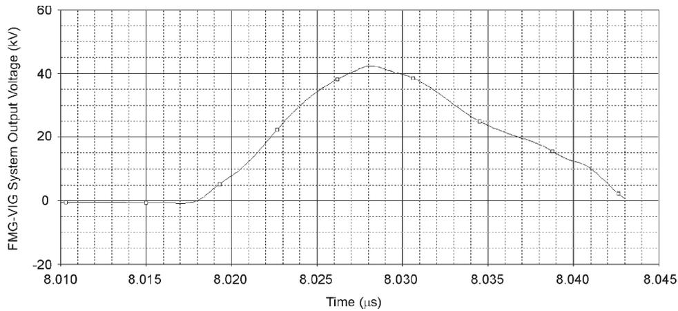
Fig. 9. Simulated waveform of the output voltage  $U(t)$  produced by completely explosive FMG–VIG system.
