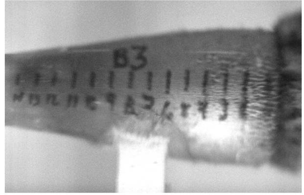
Fig. 7. Cylinder B3 during explosive expansion.
