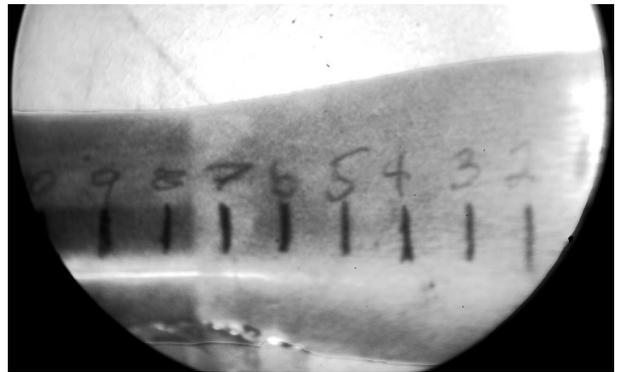
Fig. 13. Cylinder 1B during explosive expansion.
