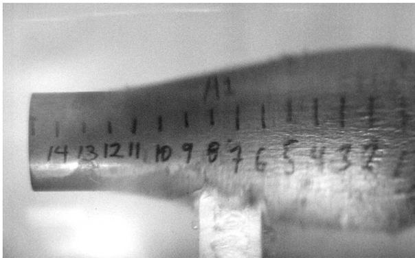
Fig. 2. Cylinder A1 during explosive expansion.
