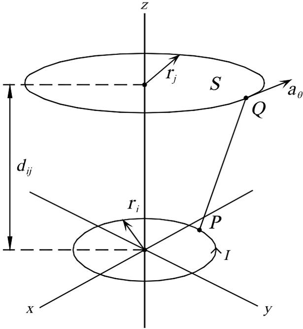
Fig. 1. Two conducting filaments, radius  $r_i$  and  $r_j$ , centred on the  $z$ -axis and separated by distance  $d_{ij}$ .
