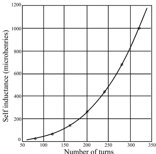
Fig. 5. Calculated self inductance of a conical inductor as a function of number of turns, measured values included.
