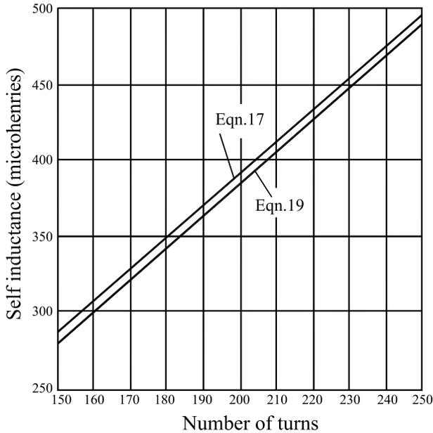
Fig. 3. Self inductance of a simple solenoid calculated using equations (17) and (19), as a function of number of turns.
