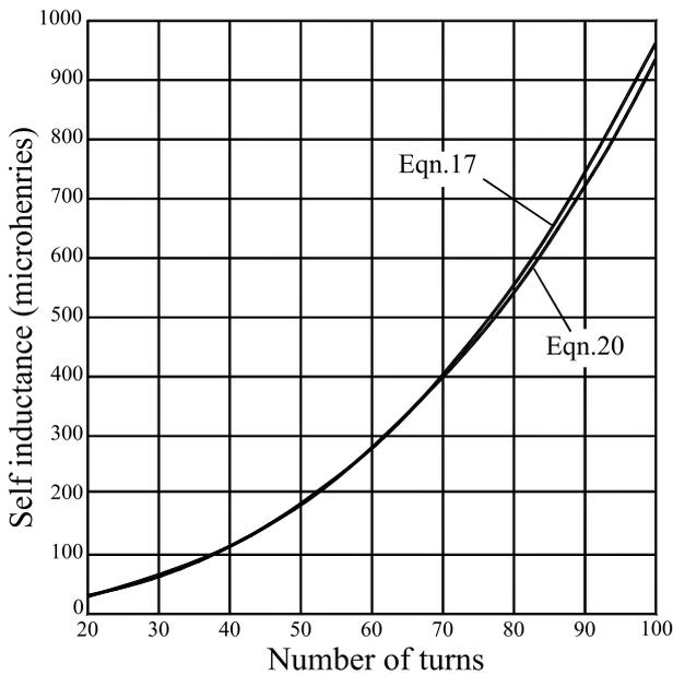
Fig. 4. Self inductance of a pancake coil calculated using equations (17) and (20), as a function of number of turns.
